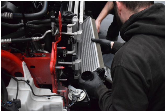
45. Remove the intercooler by lifting and tilting to release it from its mounting points.
