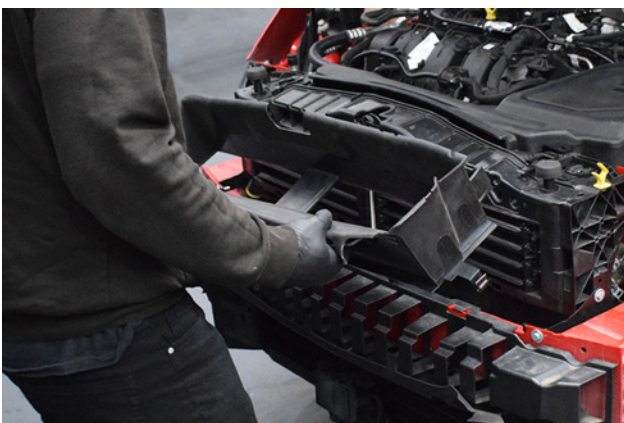
23. With the clips removed the duct can be removed.
