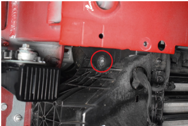
31. Remove the lower bolt located on the side of the rad pack, repeat on the other side.
