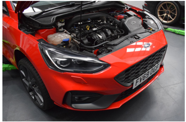
80. MVT Intercooler is now installed.
