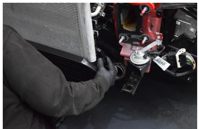
48. The bracket and mounts on the intercooler will slot into factory positions on the car.
