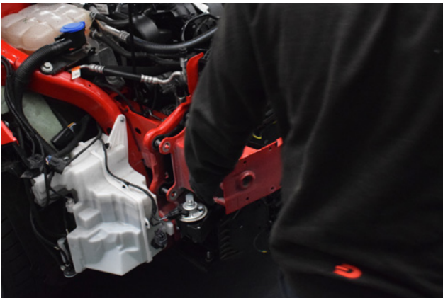
33. Carefully remove the crash bar from the car.
