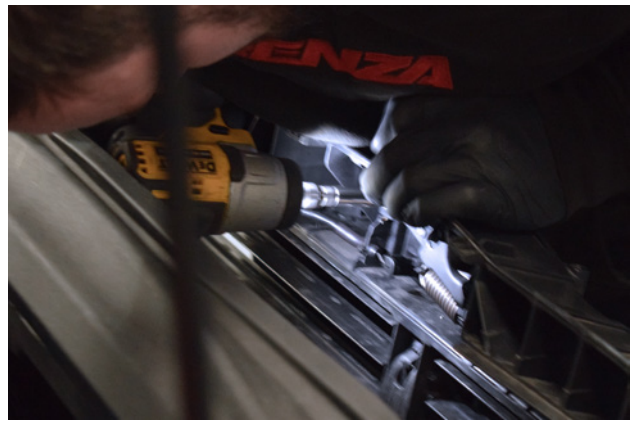
40. Behind the rad pack you will need to remove the bonnet release bolt.
