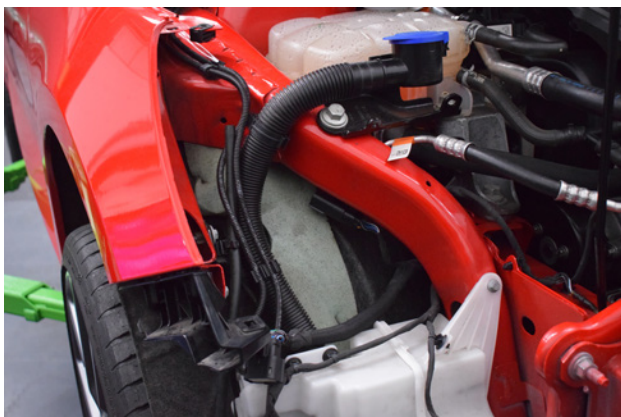
71. Re-connect and locate all sensors positioned behind the headlight.
