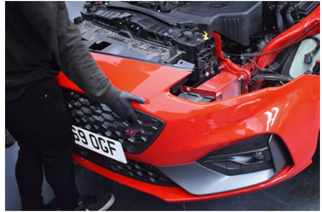
20. Carefully pull and lift away the bumper from the car.
