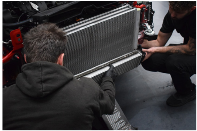
44. If you haven't already, un-clip and release the boost pipes from the intercooler core.
