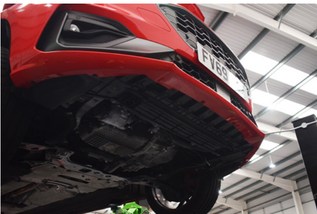
17. Raise the car in the air to access the bolts located underneath the front bumper.
