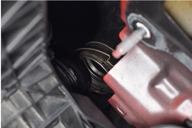
37. Use a screwdriver to release the clip on the Intercooler boost pipes.
