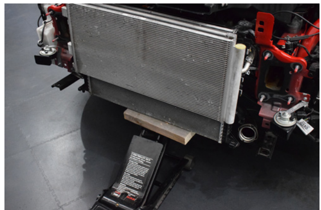
46. The intercooler is now removed.
