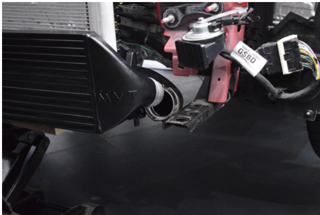
49. Once located, the intercooler will hold its weight.
