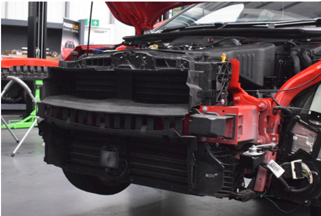
21. The front bumper is now removed.
