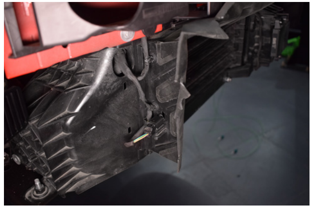
68. Re-connect the electrical sensor.
