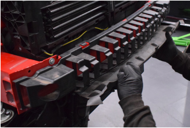
67. Install the flexible rubberized shroud onto the leading edge of the rad pack.
