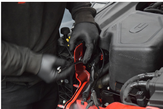
35. Remove the 2x upper bolts securing the rad pack to the car.
