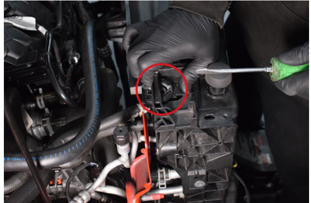
38. Squeeze the tabs on the top of the rad pack to release from the car.
