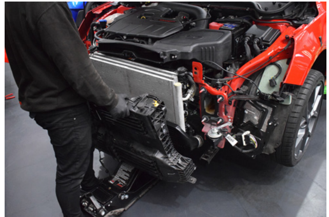
56. Carefully lift the rad pack shrouding back onto the car.
