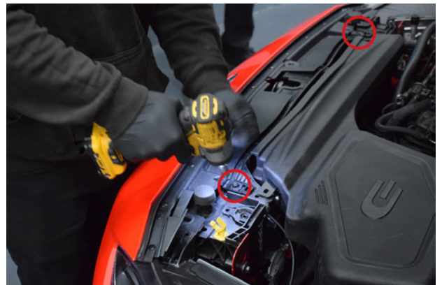
76. Slot headlight into position and secure the top mounting point with original screw..
