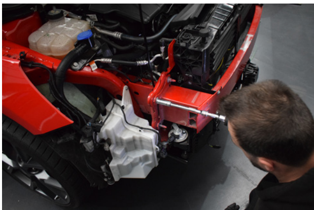
65. Tighten the crash bar using 8x nuts.
