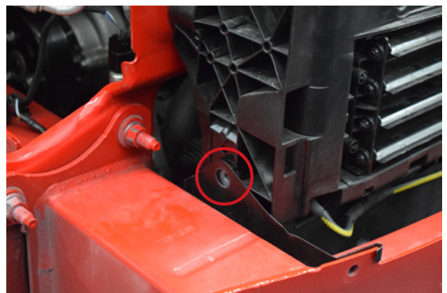
30. Remove the upper bolt located on the side of the rad pack, repeat on both sides.
