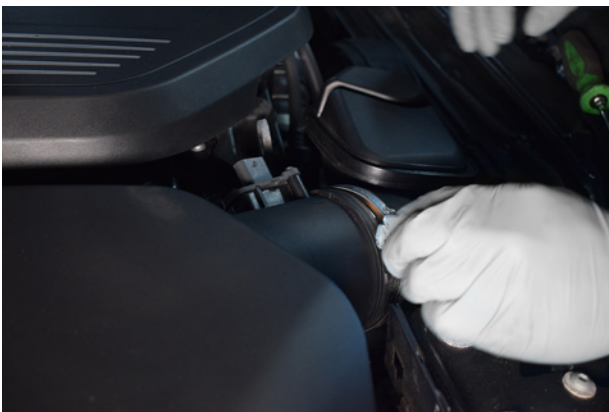
3. Separate airbox from the intake pipe.
