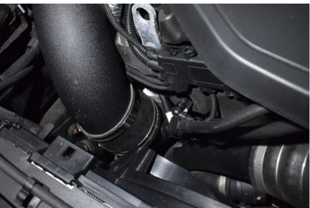
21. The Direnza intake pipe can now be installed. The exact location of the pipe will be finalised later.
