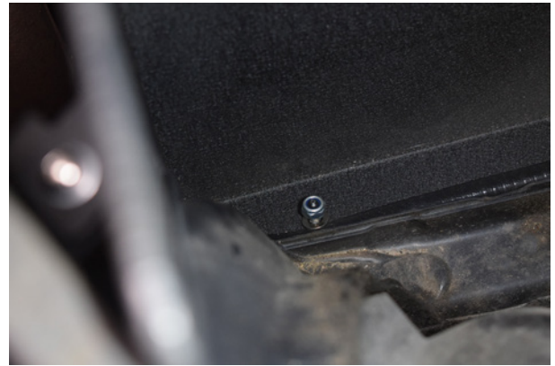
14. Secure the heat shield using supplied washer and nut.
