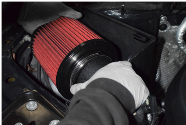
27. This step can be tricky, place the filter and jubilee over the intake pipe and over the curved section of the support bracket.
