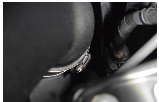
30. You can now fully tighten the 2x jubilee clips on the silicone joiner/intake pipe.
