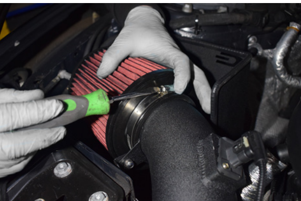
29. Secure the filter by tightening the jubilee clip.
