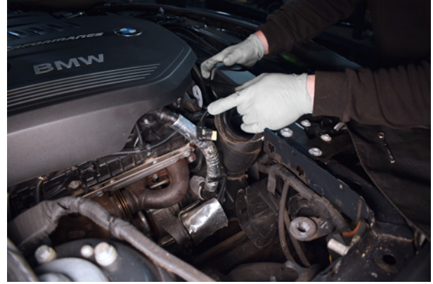
8. Remove the intake pipe.
