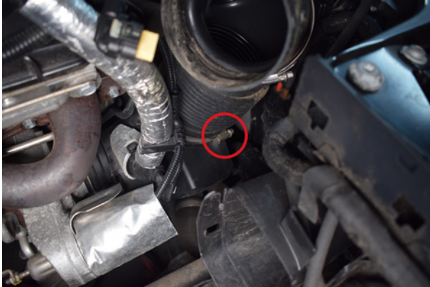
7. You can now undo the jubilee clip securing the intake pipe to the baffled intake section.
