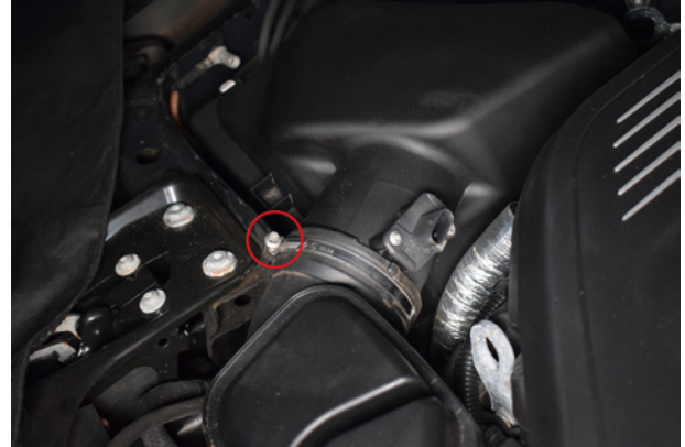
2. Undo jubilee clip securing the airbox to the intake pipe.
