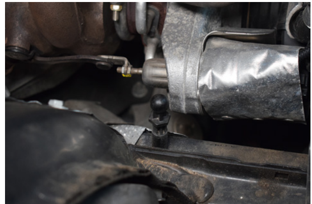
10. Remove original airbox mounting bobbin.
