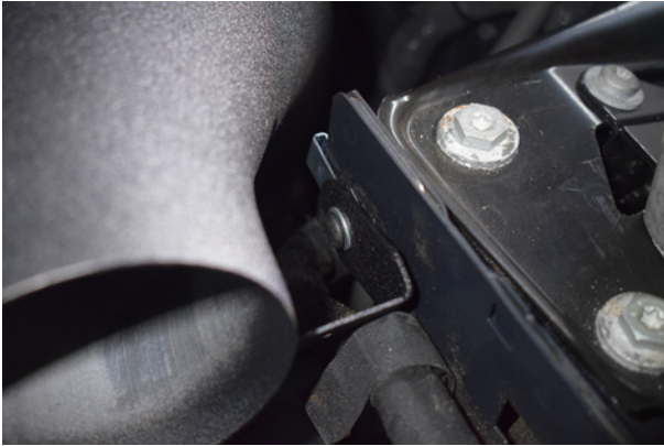
25. Secure the first support bracket using supplied washer, bolt and nut.
