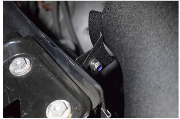
26. The second support bracket will then be secured to the first using the supplied washer, bolt and nut. Roughly positioned at the end of the intake pipe.
