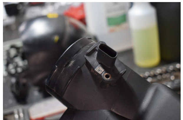
22. Remove MAF sensor mount from original intake pipe.
