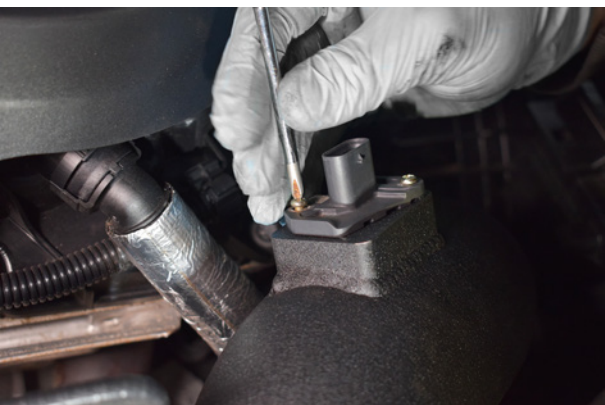
23. Install the MAF sensor mount into the Direnza intake pipe using supplied bolts.
