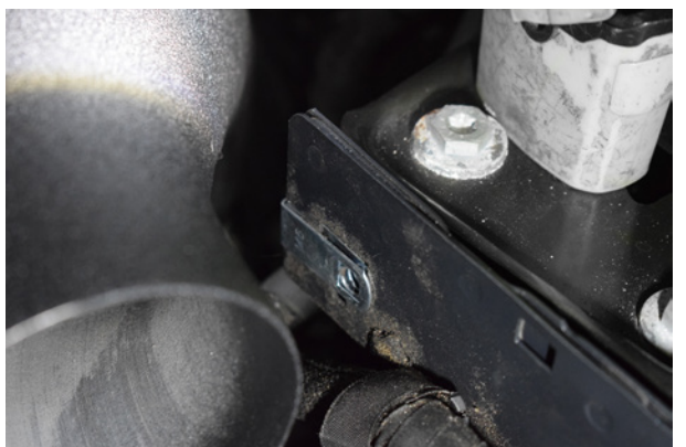
24. A second spire clip is positioned on the chassis towards the filter end of the intake pipe.
