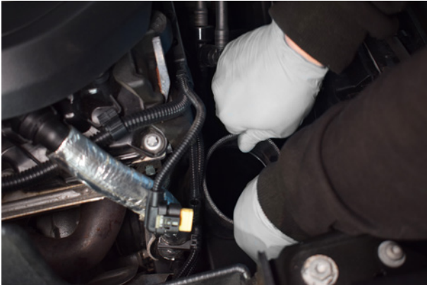
19. Install silicone joiner and 2x jubilee clips onto the baffled section of intake pipe.
