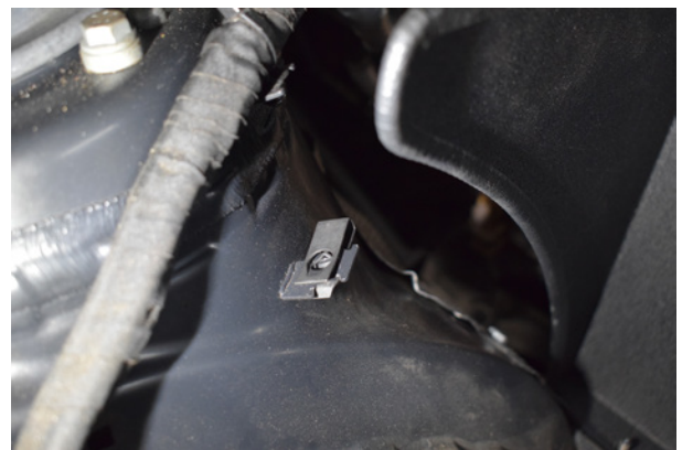
16. A spire clip is then installed on the chassis towards the rear of the heat shield.
