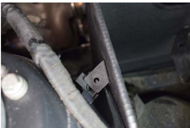
17. The mounting tap on the heat shield will line up with the spire clip.
