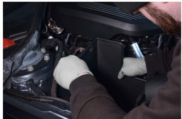
12. The Direnza heat shield can now be installed.
