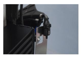
37. The sensor can be clipped into the keyhole slot on the shroud.
