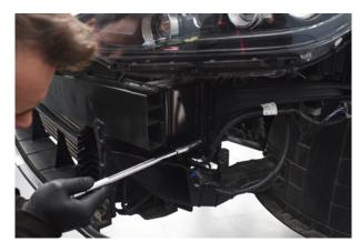
6. Remove 4x bolts securing the crash bar, repeat on the other side.
