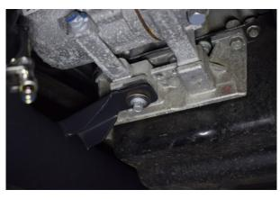
27. Don't fully tighten just yet, this will allow some movement when installing the intercooler.
