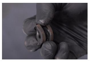
22. Remove the rubber locating grommet from the factory hard pipe and transfer onto the MVT replacement.
