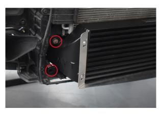
34. Lift the MVT intercooler into position and secure using 2x factory bolts and repeat on the other side.
