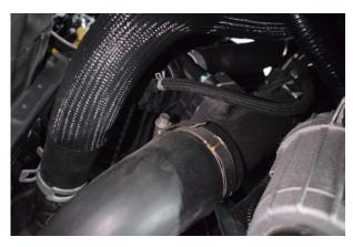
15. You can now begin removing the remaining factory boost pipes that get replaced as part of the MVT Kit.
