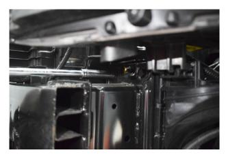
5. Remove the locating nuts on the crash bar, repeat on the other side.
