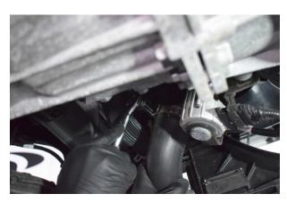
16. Remove the clamp securing the boost pipe to the throttle body.
