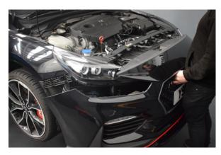
45. Install the front bumper remembering to connect the bumper loom on both sides.
