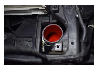
33. Place all clamps over the silicone hose in preparation for nstalling the intercooler.
