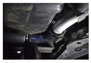
28. Nip up all clamps to hold the pipework together while allowing some movement.
