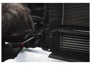
9. Unclip the wiring from the intercooler shroud.
