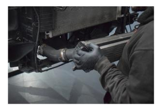
13. With the 4x bolts removed, the intercooler can be removed along with any boost pipes still connected.
