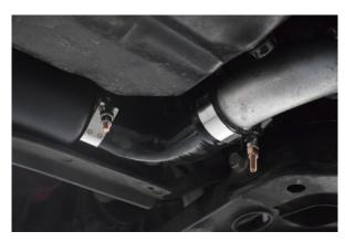
38. You can now fully tighten all hardware and clamps on the intercooler pipework.
