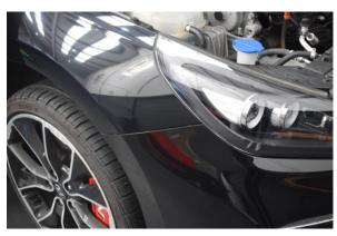
46. The edges of the bumper will clip nto position, re insert plastic clips in the wheel arch liner.
