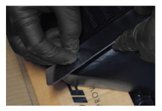
30. Off the car, install the stainless steel intercooler shroud using 4x allen bolts supplied with the kit.
