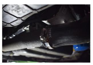
3. Undo the hose clamp that secures the rubber pipe to the hard pipe on the hot side of the intercooler.
