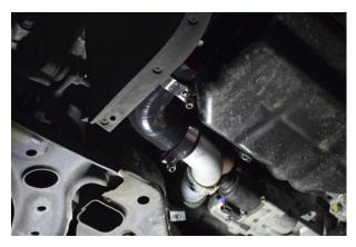
20. Install the 90° silicone joiner onto the alloy hard pipe along with two supplied clamps.
