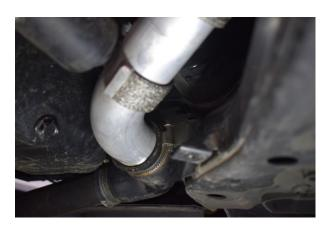
18. On the other side, remove the clamp located on the silicone positioned between the two hard pipes.
