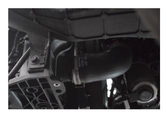
4. On the other side, remove the clamp closest to the intercooler outlet
