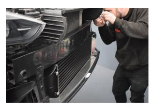
42. It will sit on the locating studs, secure the nuts on these studs first.
