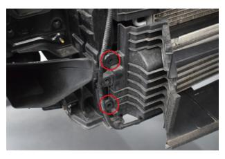
10. Remove 2x bolts securing the shroud to the rad pack.
