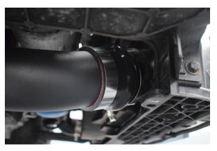
36. With the intercooler secured, you should be able to manipulate the silicone hoses over the intercooler inlet/outlet on both sides.
