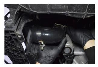
32. The second 90° silicone can be installed, this will be the join between the throttle body and MVT.
