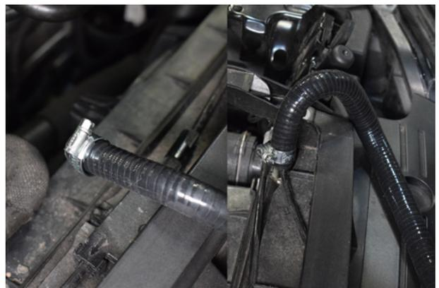
18. Before installing the replacement water pipe, place the small jubilee clamps on the end.
