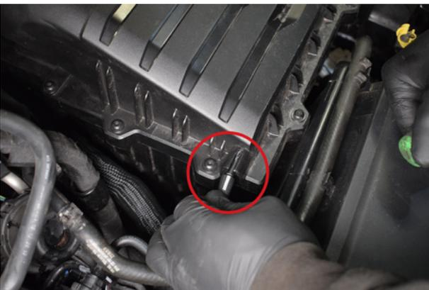
5. Remove the vacuum pipe from the standard airbox
