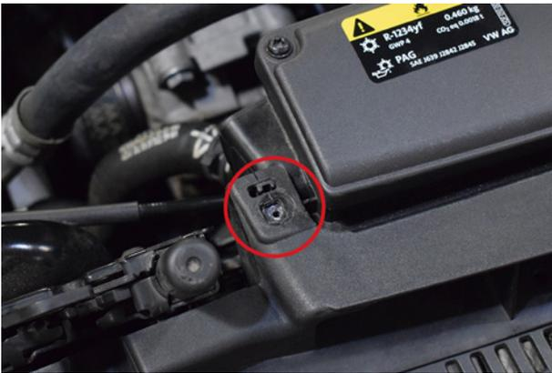
3. Remove 2x screws on the front panel.
