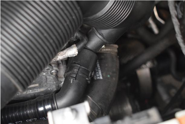
7. Remove the recirculation pipe from the intake assembly pipe.
