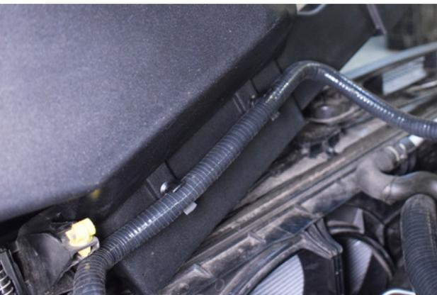
35. As you place the airbox into the engine bay, clip the water pipe into the fir-tree clips.
