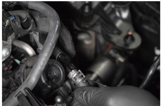
16. Undo 2x clips at both end of the water pipe and remove.
