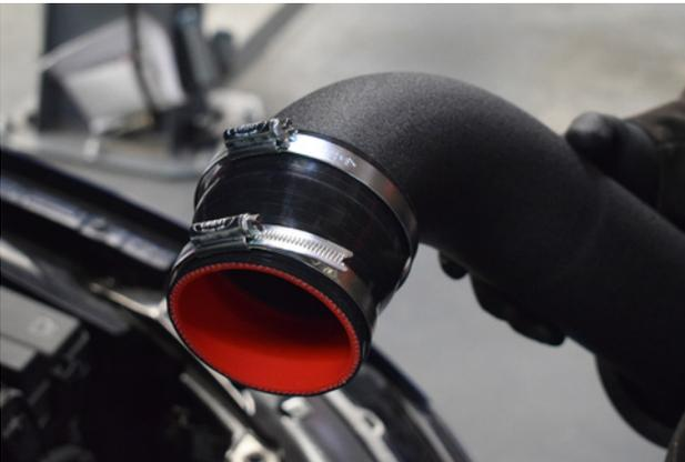
33. Place a silicone reducer on the other end of the air pipe and secure using supplied clamps.
