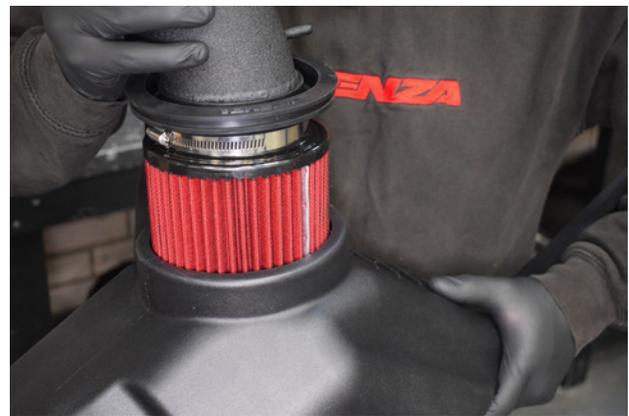
34. Place the filter assembly inside the Vortex Airbox. The rubber Pro Flex Seal grommet will secure everything in place
