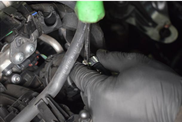
21. Secure the water pipe by tightening the jubilee clamps with a screwdriver.
