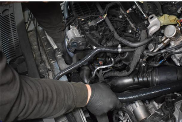
23. The replacement recirculation pipe can now be installed.
