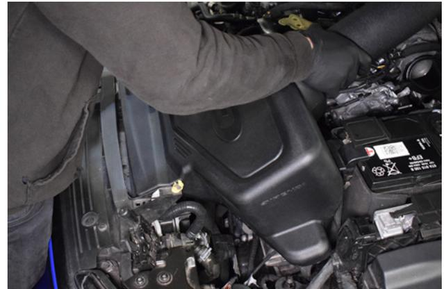
36 Continue to lower the airbox into the engine bay, the rubber grommet will secure into the original mounting bobbins.
