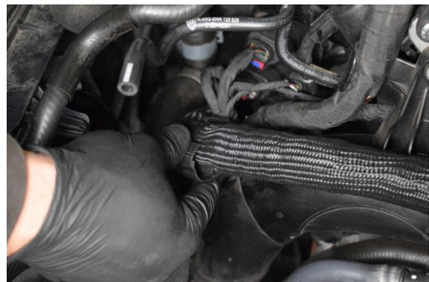
12. Remove recirculation pipe from the plastic containing clip.
