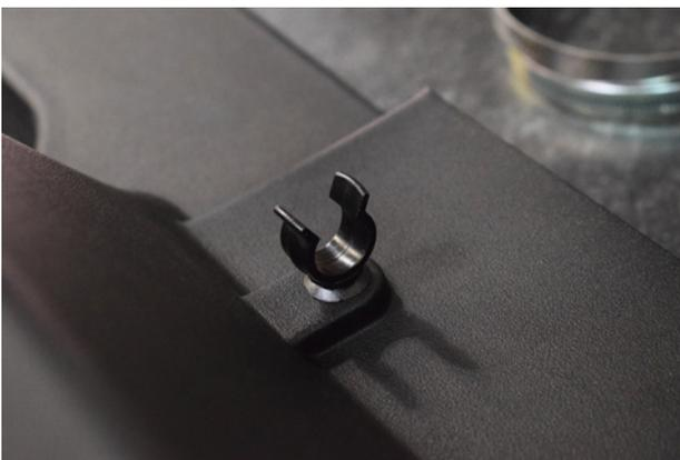
29. Insert 2x Fir-tree clips into the underside of the airbox.
