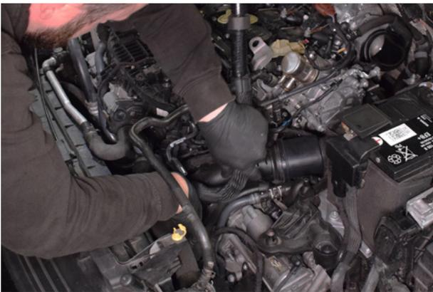
15. Once released, remove recirculation pipe from the car.
