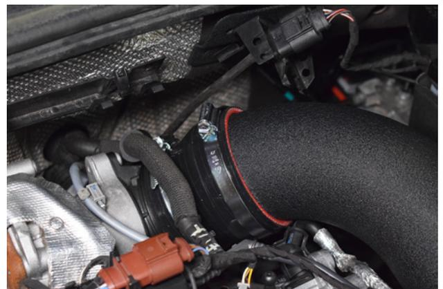
42. Ensure all jubilee clamps on the silicone reducer are appropriately tightened.
