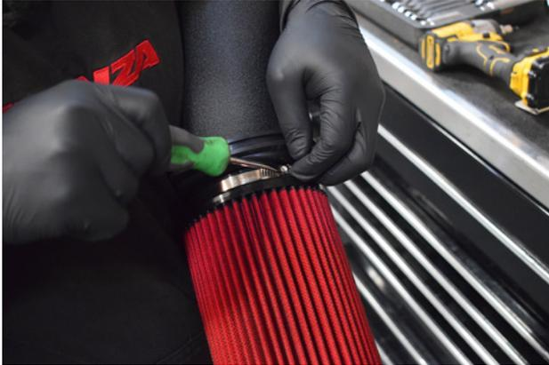
31. Place the Air Filter & Pro Flex Seal onto the air pipe. Secure the filter to the air pipe using the supplied clamp
