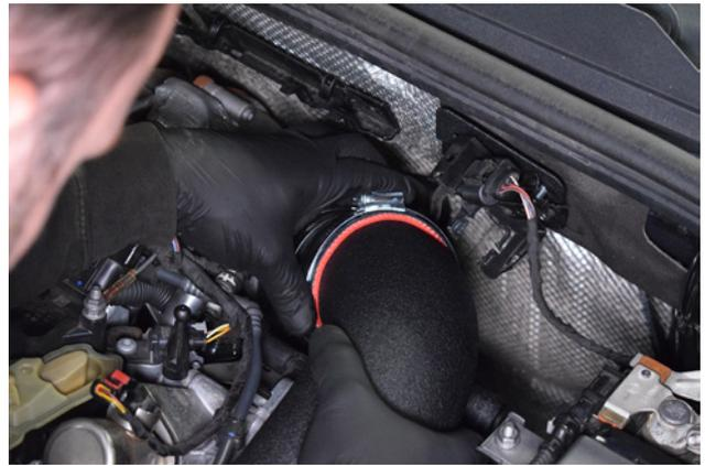
38. Place the silicone reducer onto the turbo inlet.
