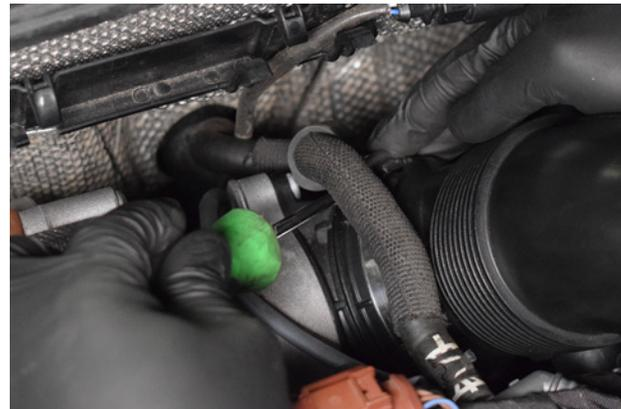
6. Undo the clip securing the intake pipe to the turbo inlet.
