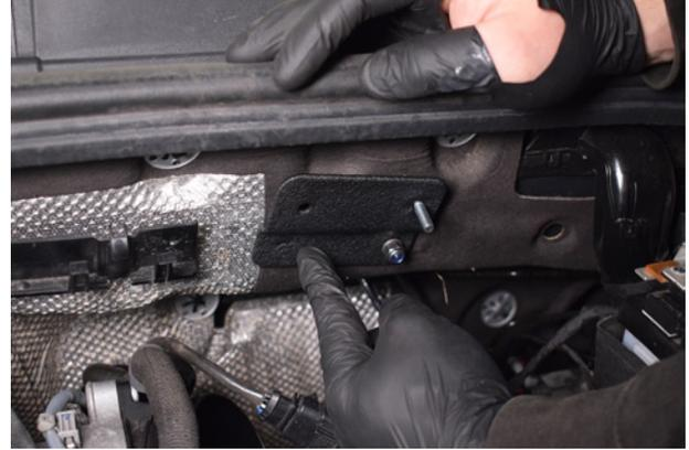
26. Place the 'Z' bracket onto the bulkhead as pictured.
