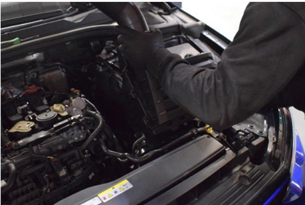
9. The airbox assembly can now be removed from the car.
