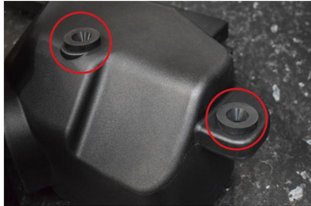
28. Insert 2x rubber grommets into the underside of airbox.
