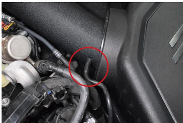
41. Re-insert factory vacuum pipe into the air pipe.
