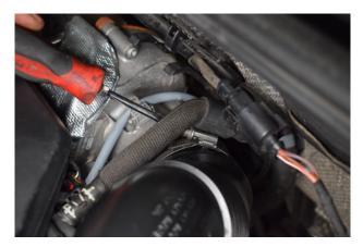
2. Undo the jubilee clip securing the intake pipe to the throttle body.
