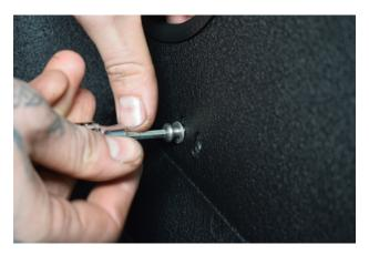
25. Fasten the Airbox to the Airbox bracket using 2x supllied bolts and washers
