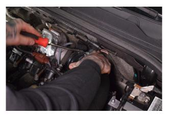
21. Using a flathead screwdriver, tighten the 2x jubilee clips on the silicone reducer.
