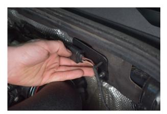
20. The lambda sensor and bracket can then be relocated away from the intake pipe.
