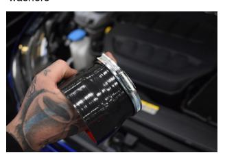
27. Place jubilee onto silicone reducer and place onto the throttle body.
