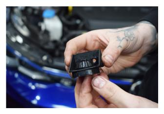
19. The third bobbin is installed on the Airbox support bracket.
