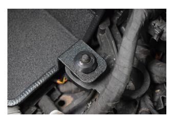
23. Ensure the bobbins are securely mounted on the OEM mounting points.
