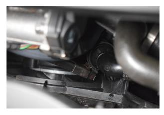
10. Using a spring clip tool, undo the clip securing the recirculation pipe to the recirc valve.
