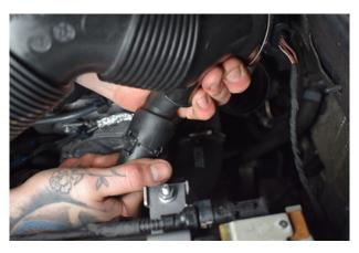
6. This allows the intake pipe to be lifted and the recirculation pipe removed.
