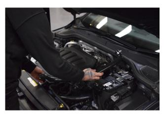
15. Place into the car, installing the lower end of the pipe onto the recirculation valve.
