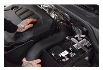
20. You can now slide the intake pipe into the silicone reducer and lower into the correct position.
