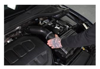
7. The OEM Airbox assembly can now be removed.
