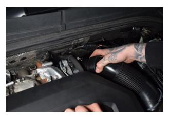
3. Once loose pull the intake pipe away from the throttle body to release.
