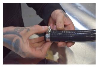
13. Place a jubilee clip on each end of the silicone recirculation pipe suppled in the kit.
