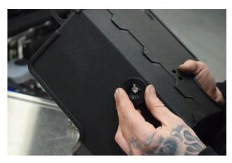
17. Install 2x Polyurethane bushes into the Airbox.
