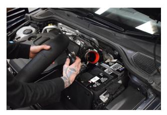
25. Push the remaining end of the recirculation pipe onto the Direnza intake pipe.
