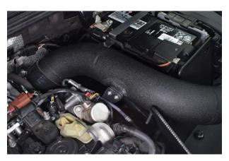
23. Install supplied bolts and washes to secure the bracket to the intake pipe.
