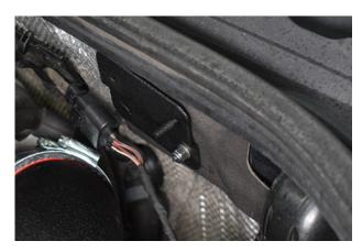
19. Install bracket on OEM stud and secure using supplied nut.
