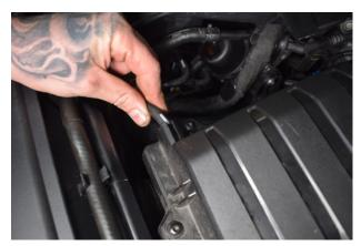
4. Remove the vacuum line from the OEM Airbox.
