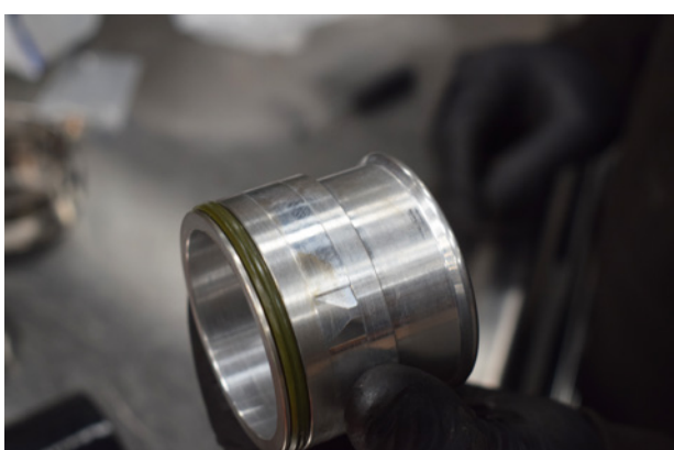
70. Install the O ring onto the new adapter.
