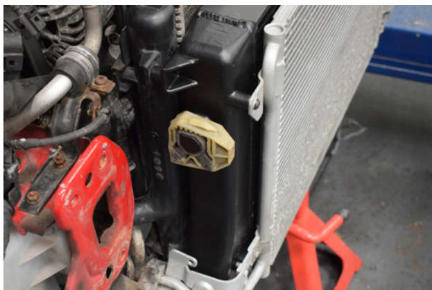
55. Re-install the plastic clips onto the intercooler.
