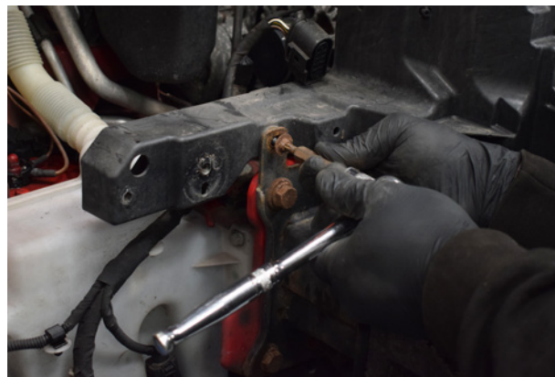
14. Remove the upper and lower screws from the crash bar.
