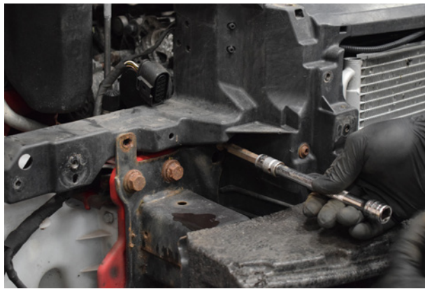
16. Undo additional screws on the cooling shroud.
