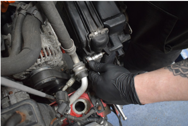
43. Remove the upper screw securing the intercooler to the rad pack and repeat on the other side.
