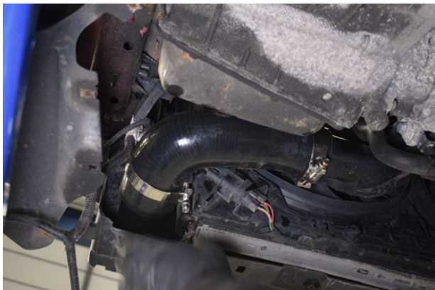
72. Place the supplied clamps onto the 90° silicone and install.
