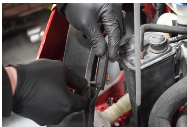
32. Disconnect the bonnet release cable.
