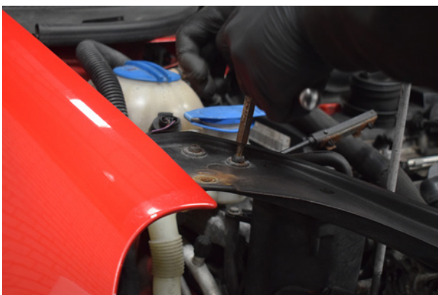
35. Remove 2x screws on the slam panel and repeat on the other side.
