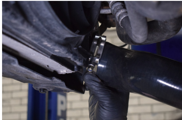
74. repeat this process for the boost pipe on the other side of the car.
