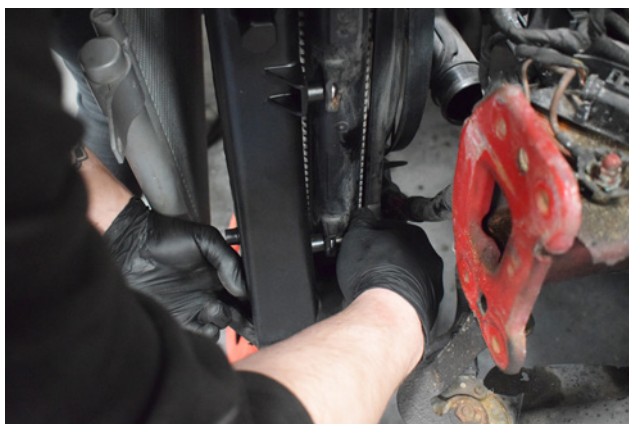
49. With the mounting points lined up with the rad pack you can secure the intercooler using the supplied hardware.
