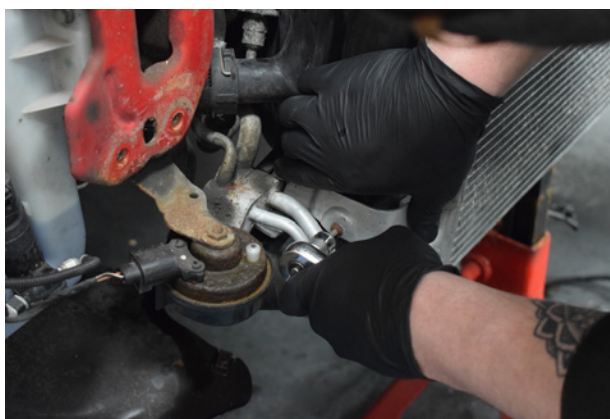
42. Remove the final screw located on the side of the condenser, it can then be safely held out of the way.
