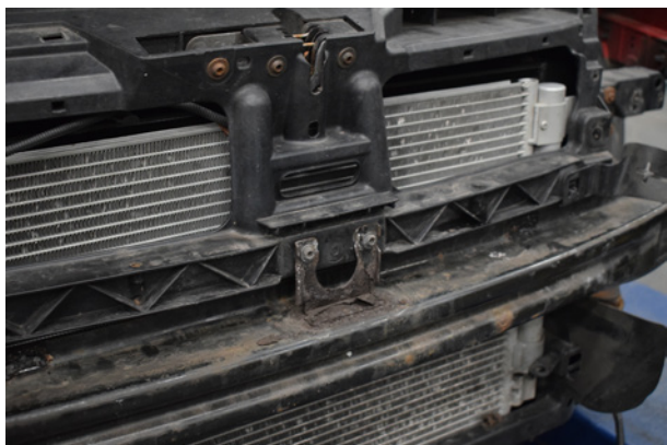
67. Re-install the two central locating screws on the crash bar.
