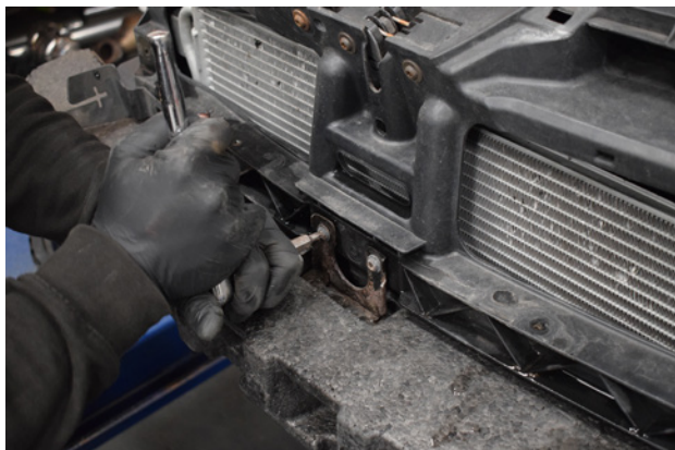
13. Undo 2x screws from the centre of the crash bar.
