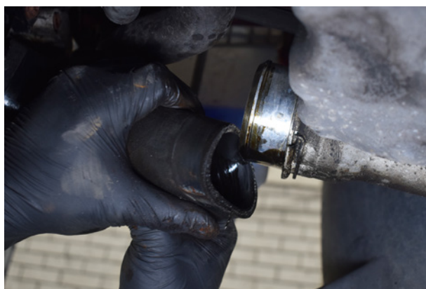
22. With the clamps released, you can remove the OE silicone pipes.
