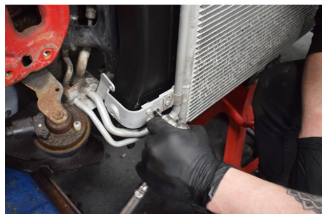
53. Not forgetting the final screw next to the air con pipes.
