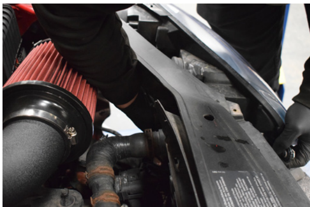
7. Disconnect the headlight plug before removing.
