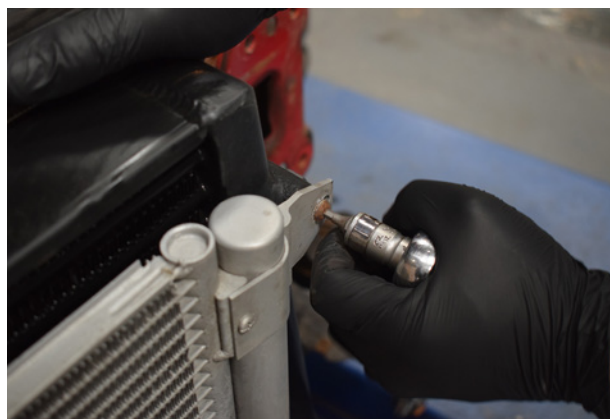
40. Remove screw securing the condenser to the intercooler.
