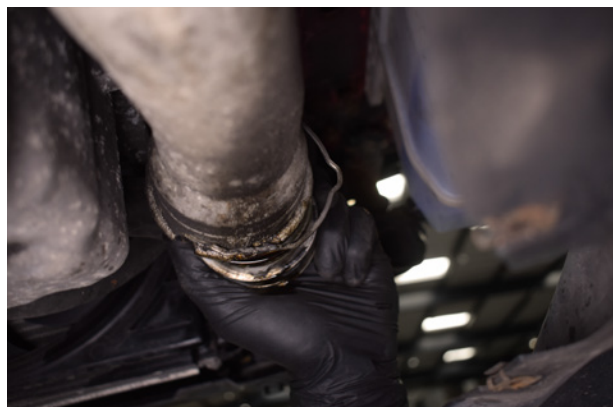
68. Remove the boost pipe adapter from the hard pipe.
