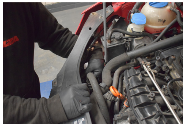
60. Reconnect the bonnet release cable and bonnet detection sensor.
