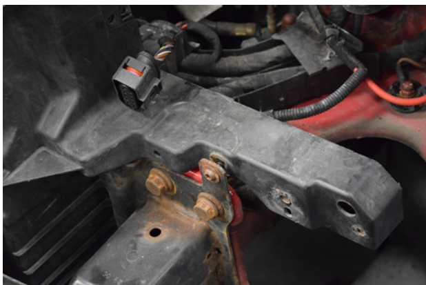
65. Install smaller crash bar mounting screws.
