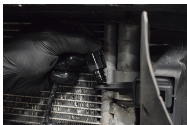
12. Remove air temperature sensor.
