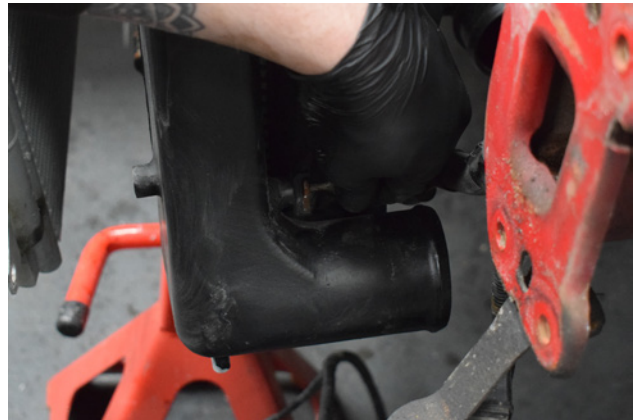
44. Remove the lower screw securing the intercooler to the rad pack and repeat on the other side.
