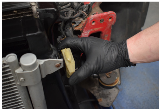
38. Remove the plastic clip from each end of the intercooler.
