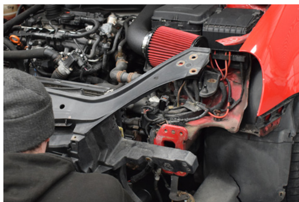
56. The plastic slam panel can now be re-installed.
