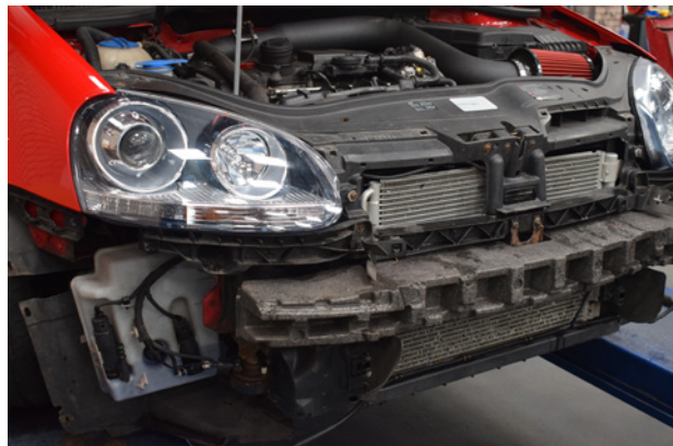
76. With the intercooler installed you can re-fit the front bumper.
