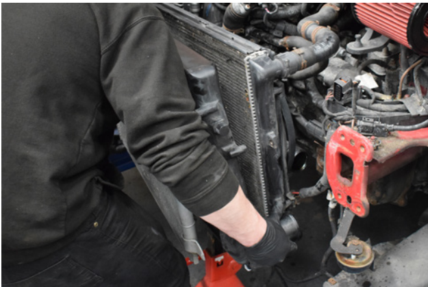
45. The intercooler can now be removed from the car..
