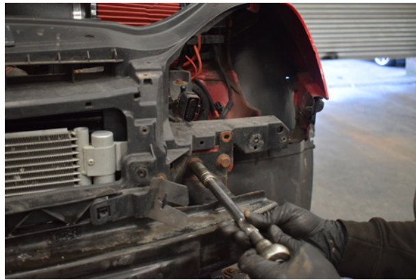
26. You can now undo the 4x bolts securing the crash bar to the chassis.
