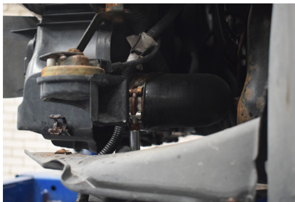
18. Undo 4x clamps on the intercooler boost pipes.
