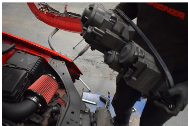
9. Remove the headlight and repeat the removal process on the other side.
