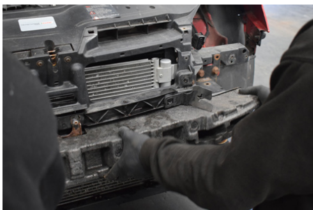
17. Remove the polystyrene crash bar cover.
