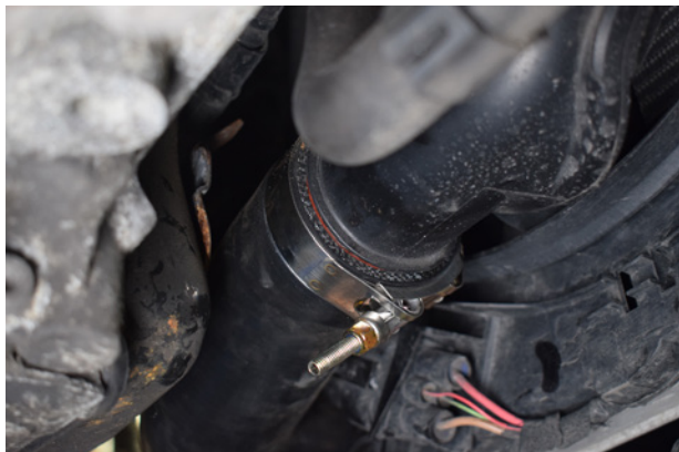
73. Tighten clamps to secure.
