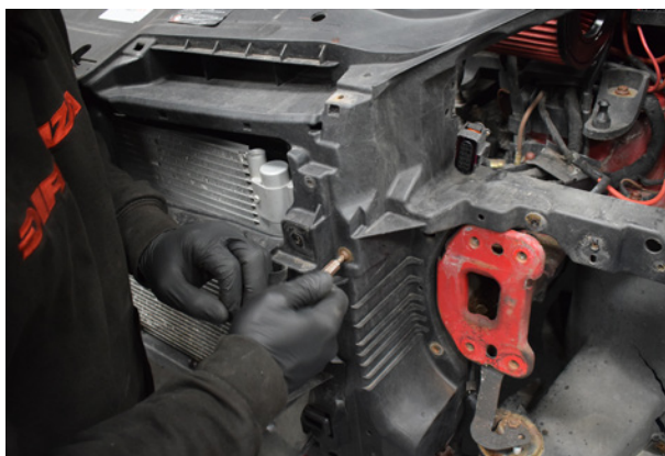
36. Remove the final 2x screws hidden behind the crash bar.
