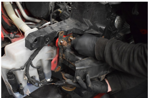
63. Secure the crashbar using 4x original bolts and repeat on the other side.
