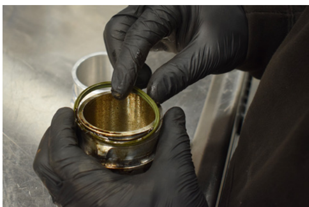
69. The O ring needs to be transferred to the supplied adapter.
