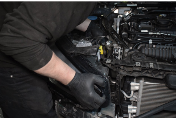
29. With all the bolts removed, the headlight can be lifted out of position.
