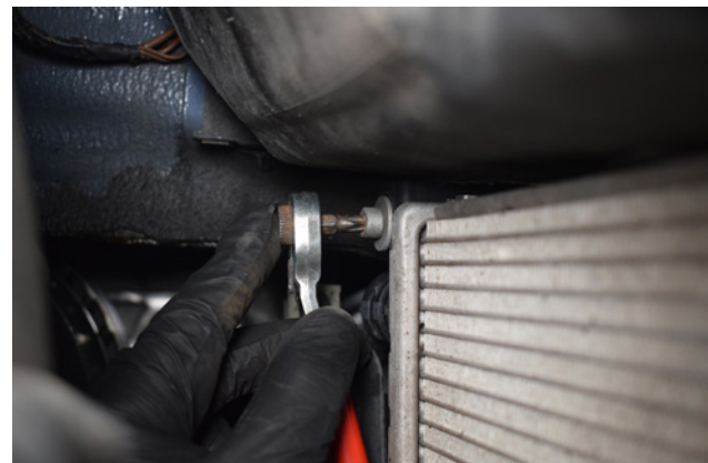
18. Remove the bolt from the top corner of the side mount radiators. Repeat on both sides.
