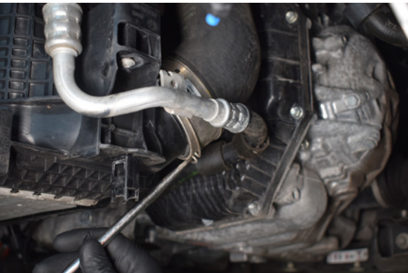
51. Unclip the the boost hose from the intercooler.
