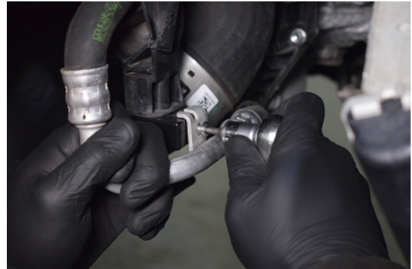
62. Reconnect the Air Con bracket to the intercooler.
