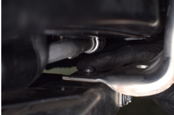
85. Install lower mounting screw on the support bracket located underneath the scoop.
