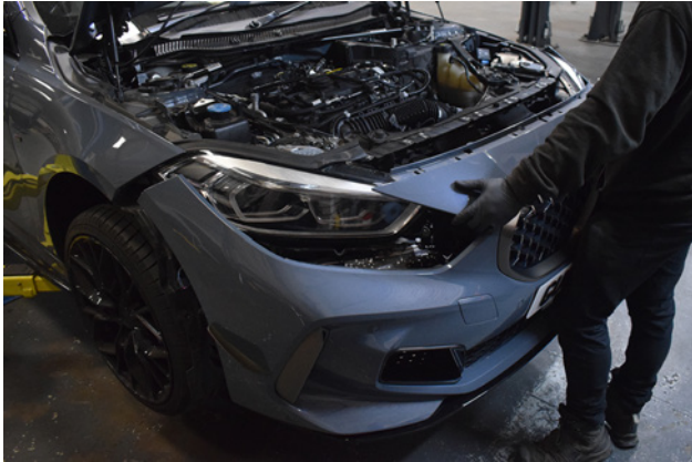
1. Remove the front bumper.
