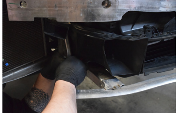
86. Install the support bracket on the other side and repeat previous steps for installation.
