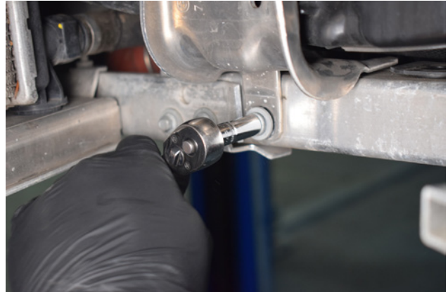
14. Remove the bolt from the lower subframe assembly, repeat on both sides.
