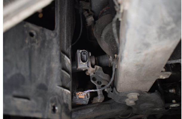
44. Unplug headlight leveling sensor.
