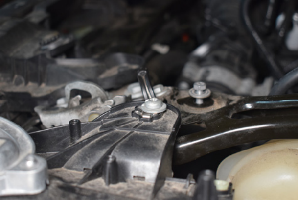
25. Remove top headlight mounting bolt.
