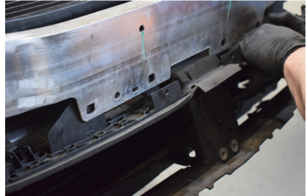
72. Install the second ducting panel by clipping it into position on the crash bar.
