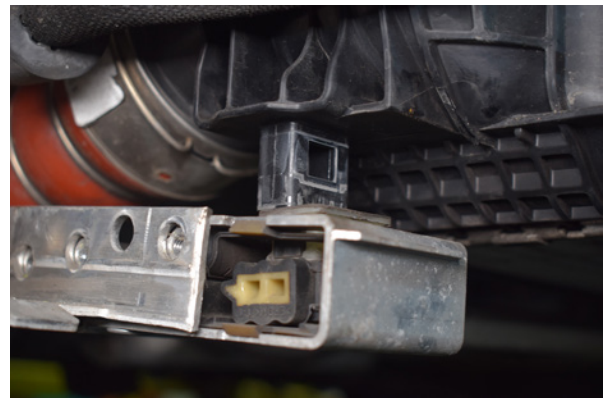
48. Simultaneously lift the intercooler and drop the support frame to release from each other.
