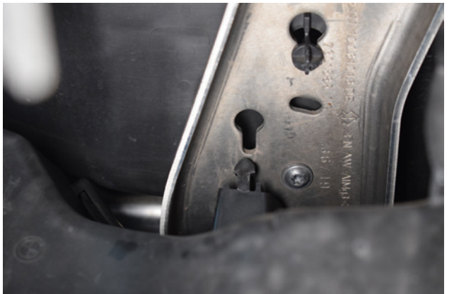
6. Lift the scoops from either side of the car and pull out from keyhole slot in the brackets they are connected to.
