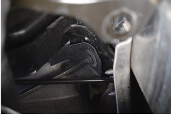
97. The radiator scoop is secured with 1x screw on each side.
