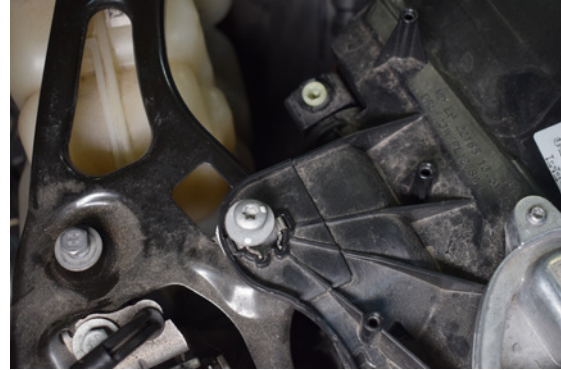
110. Secure headlight with all original hardware.
