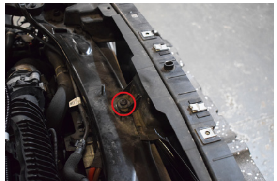
106. Plus one central torx screw
