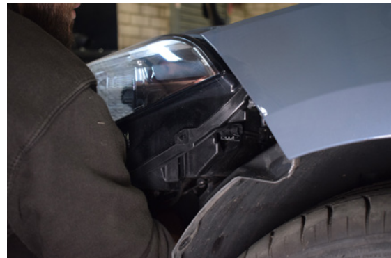
112. The final mounting screw is located in the wheel arch.
