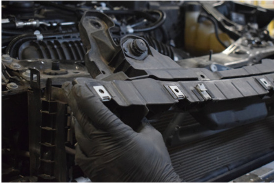
103. Place the plastic slam panel back into position.
