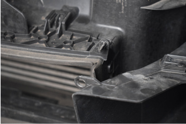
7. Pull the scoops forward to release them from the plastic pin on the front cooling shroud.
