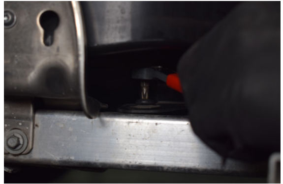
88. Secure the plastic scoop using a T25 torx and repeat on the other side.
