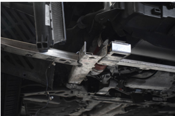
65. Slide the lower subframe assembly into subframe.
