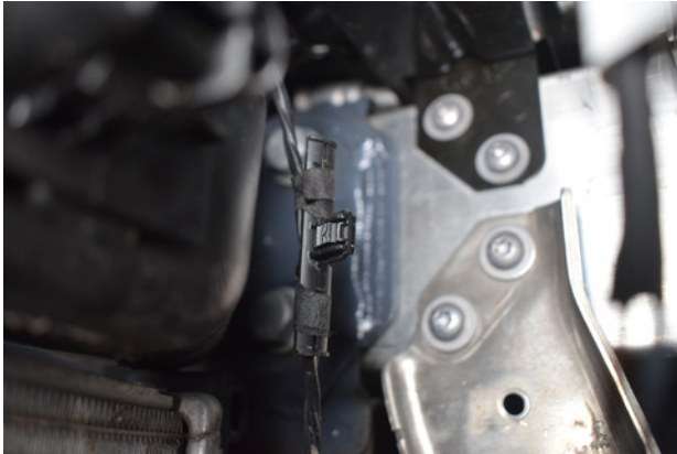
19. Remove any plastic clips or wiring from the bracket.
