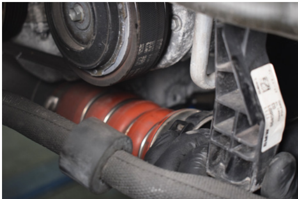
57. Push the boost hoses over the inlet/outlets on the intercooler. You will hear a popping noise as they clip into place.
