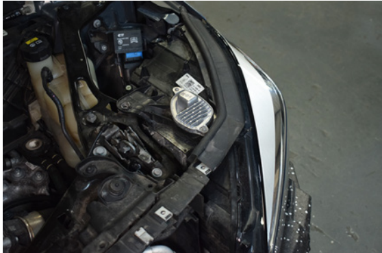
109. Place the headlight into position.
