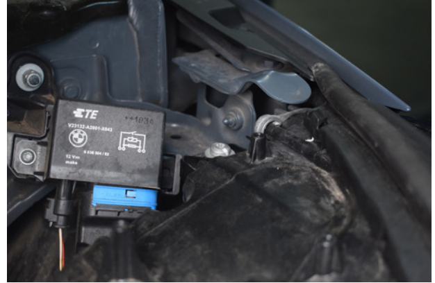
26. Remove the most rearward headlight mounting bolt.
