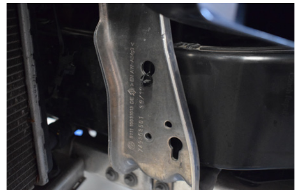
84. The scoop clips into the keyhole on the support brackets.
