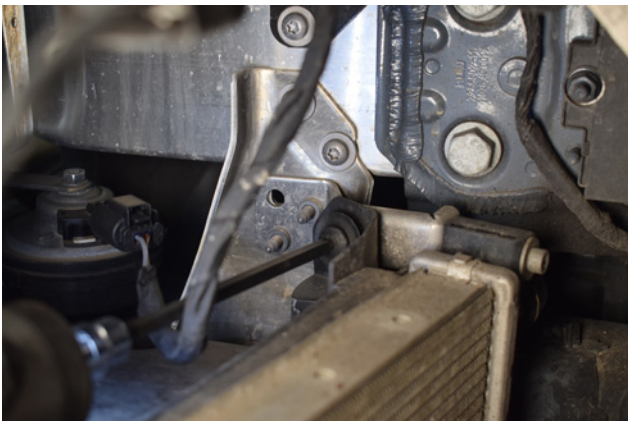
11. Remove the screw securing side mounted radiator air scoops.
