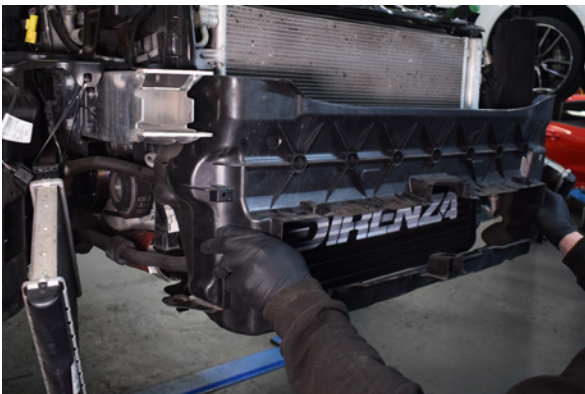
63. Place the intercooler ducting into position on the car.
