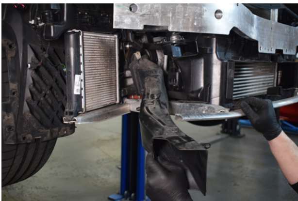
21. With the bracket out of the way, the brake cooling duct can now be removed.
