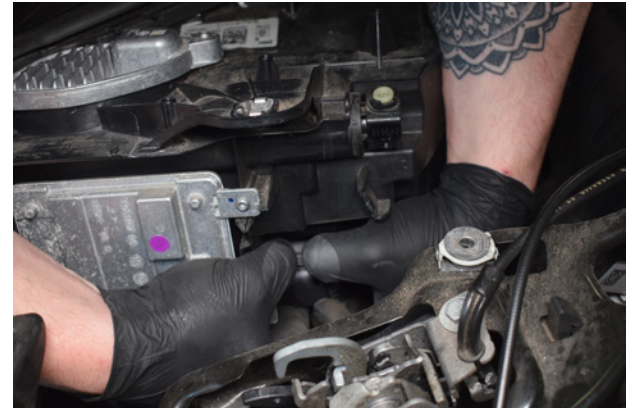
30. Before removing completely, ensure all plugs and wires are disconnected from the back of the unit.
