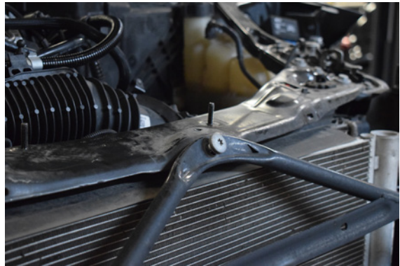
100. Install front brace using 3x Torx screws.
