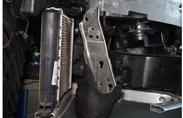
20. You can now remove the support bracket.
