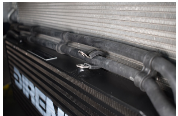
60. Place the 'C' clips around the pipes that sit above the intercooler.
