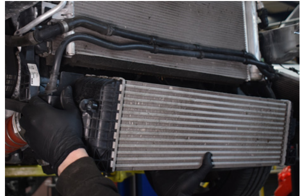
54. The intercooler can now be removed.
