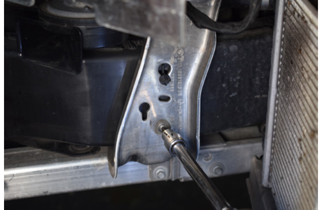
10. Remove 1x screw from the bracket located either side of the car.
