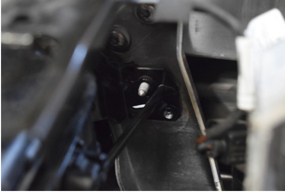
79. A further mounting bolt has to be installed from the rear of the bracket.
