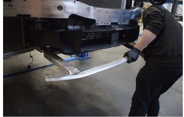
74. Slide the second piece of the lower subframe assembly back into position.
