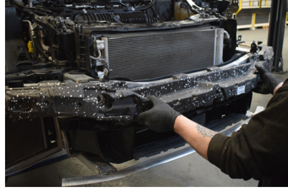
92. Install the polystyrene onto the crash bar
