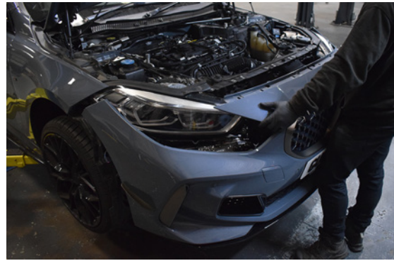
116. Re-install the front bumper.
