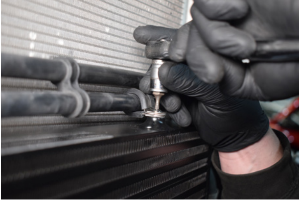
61. Squeeze the clips together and secure to the intercooler.
