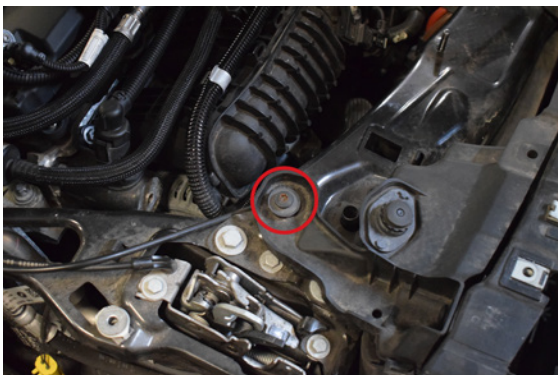
105. The plastic panel can be secured by installing torx screws on each side.
