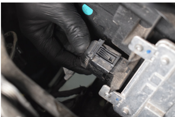
107. Plug everything in on the rear of the headlight unit.
