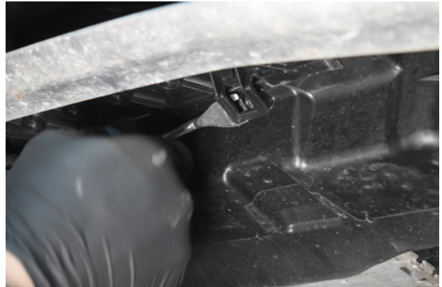
8. Lift up x4 tabs on the shroud to release it from its mounting points.
