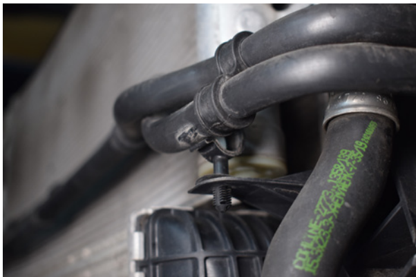
41. Unclip all pipework connected to the intercooler
