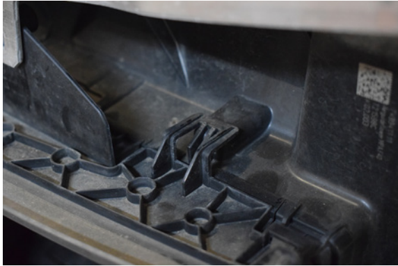
73. The tabs will slide over clips on the first ducting panel you fitted.
