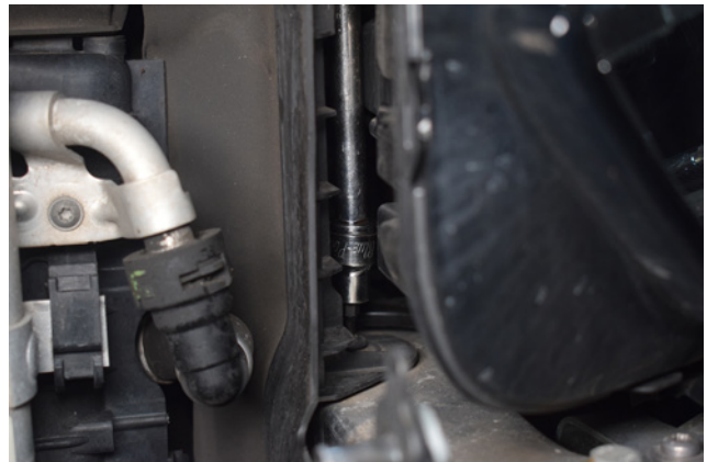
12. Undo the second screw and remove the scoop. Repeat on other side.
