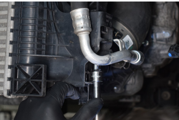
53. Remove the final screws securing the intercooler to the car, repeat on both sides.
