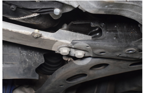
46. Remove 2x bolts securing subframe assembly to the subframe. Repeat on the other side.
