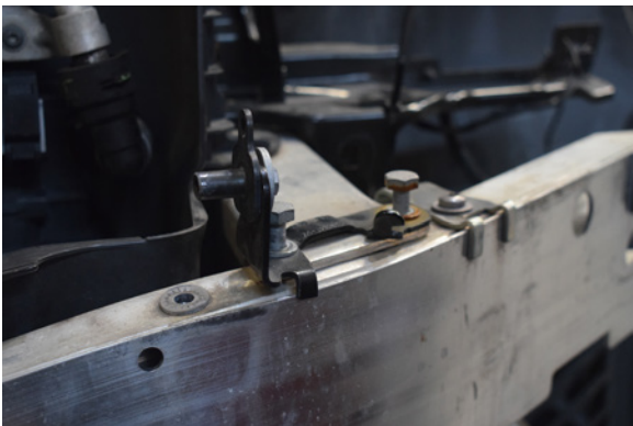
69. Re-Install the crash bar brackets x2
