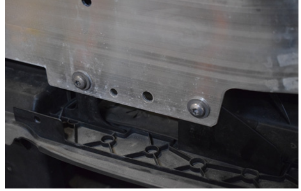
80. Install 4x screws into the crash bar.
