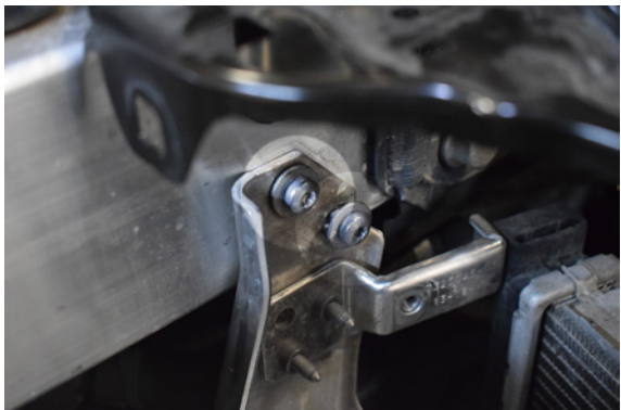
77. Insert a further two screws into the side bracket to fix to the crash bar.
