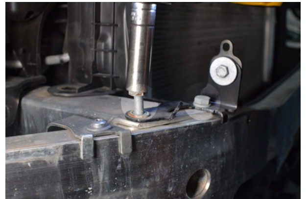
36. Remove bracket from the top of the crash bar by removing 2x bolts.
