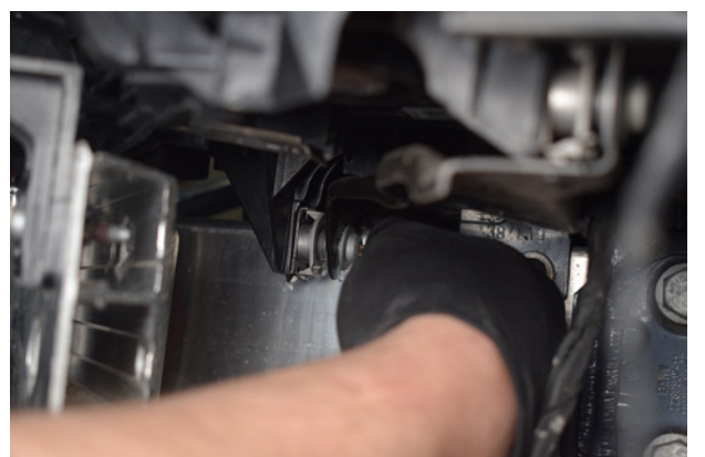
24. Remove headlight bolt located underneath in the wheel arch.
