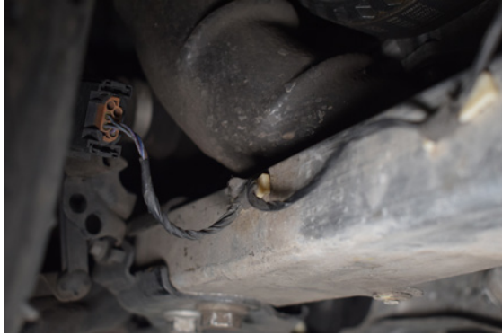
91. The wire for the sensor clips in down the side of the subframe assembly.
