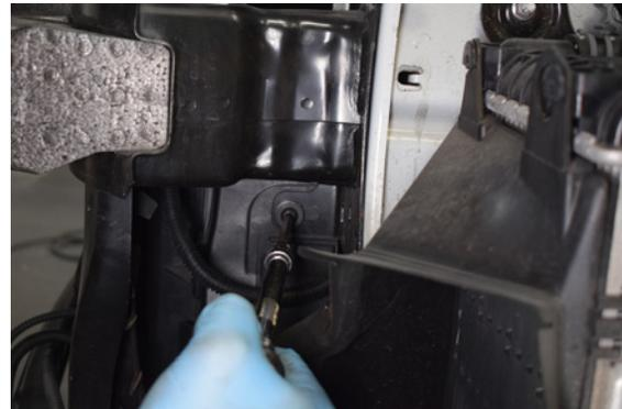
56. Undo additional 2x torx screws on the crash bar plate.
