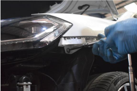
43. The final screw is located on the side below the front wing.
