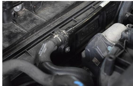
66. Undo the 2x screws securing the water pipe.
