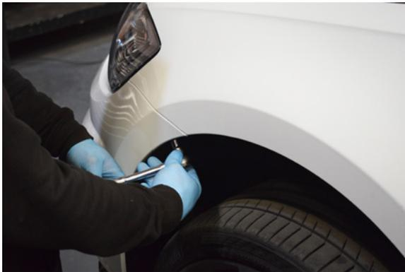
21. Repeat the process on the other side to release the front bumper,
