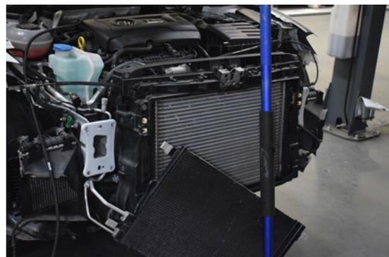
70. The condenser can hang safely out of the way.
