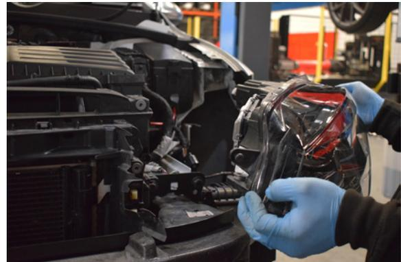
44. With all three removed you can lift the headlight away from the car.
