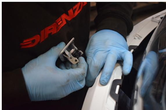
29. The cover unclips allowing you to remove the bumper.
