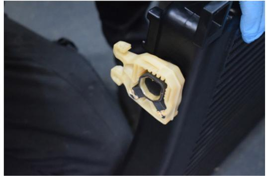
76. Remove the plastic retaining clips from the OEM intercooler and install onto the Direnza MVT.
