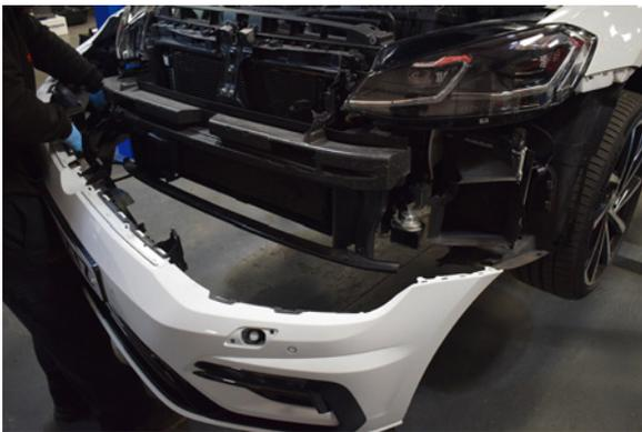
33. Before removing you will need to unclip lower wiring from the bumper.
