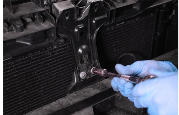
38. Remove 4x screws on the upper rad pack bracket.
