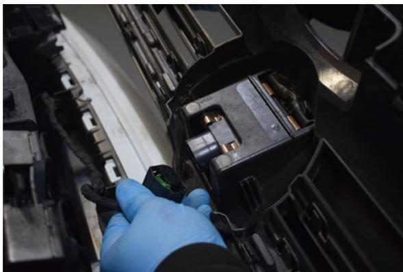
13. Disconnect the motion detector radar.
