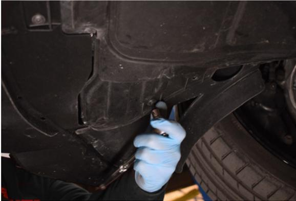
19. Remove screw securing the engine undertray & repeat on the other side.
