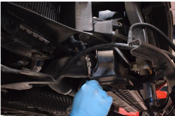
47. Undo the Jubilee clip on the intercooler boost pipes.
