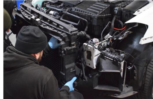
80. This frame is fitted using the plastic clips attached to the intercooler.
