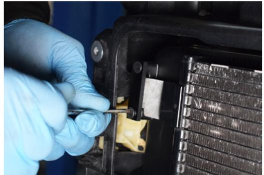
84. Secure the condenser with the supplied retaining brackets and hardware.
