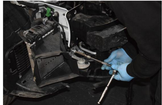
52. Undo bolt securing the horn.
