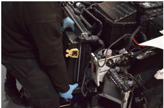
77. The intercooler can now be lifted back into position.
