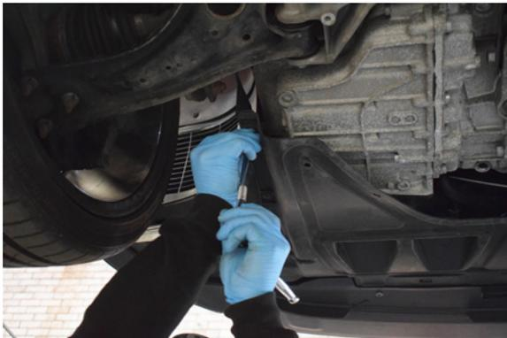
23. Undo remaining engine undertray screws to free it from the car.
