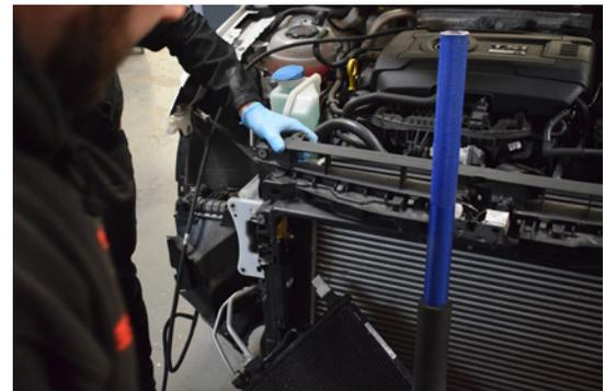
72. With the clips pressed and released, remove the plastic frame.
