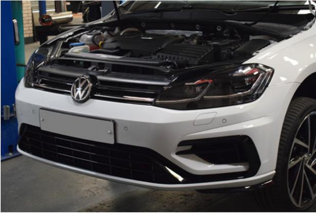
1. Open the bonnet and lift the car. If using a Jack place the car on Jack Stands once raised high enough.
