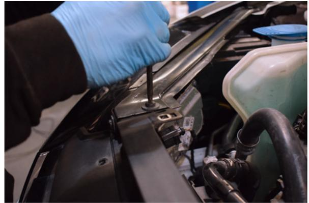
8. Remove 2x screws securing the metal trim piece.
