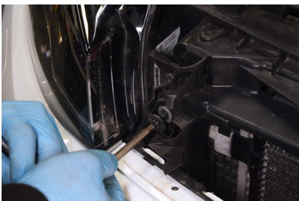
15. Remove further 2x bumper screws (1 each side).
