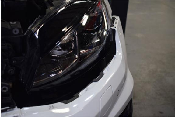
31. Remove the headlight washer cover on the other side of the vehicle.
