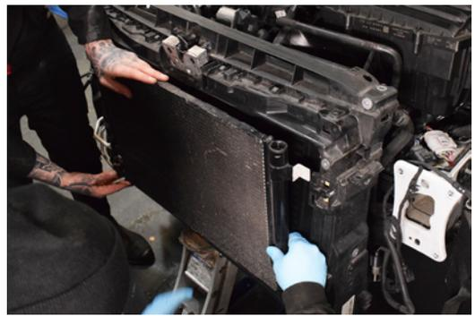
82. The condenser can now be lifted into the securing tabs on the MVT intercooler.
