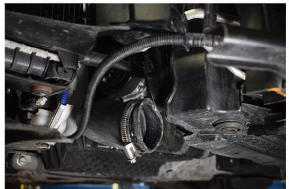
48. Remove the boost pipes from the intercooler.
