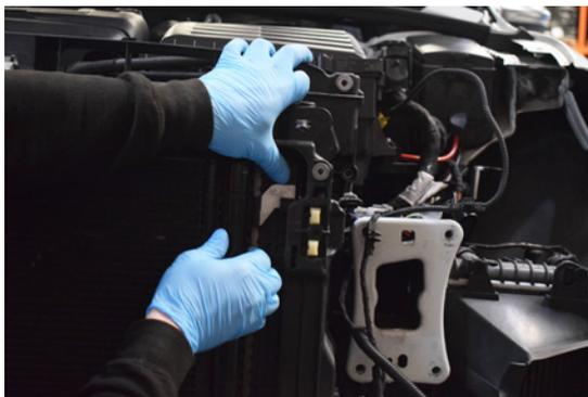
69. Lift the condenser so that the locating tabs are lifted above the retaining clips.
