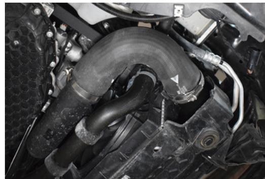
90. Push the OEM boost pipes over the MVT intercooler end tank inlet.
