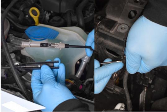
61. Unclip any wiring attached to the rad pack.
