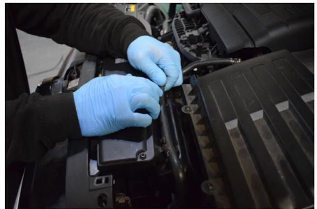
4. Remove the breather hose from its retaining clips.
