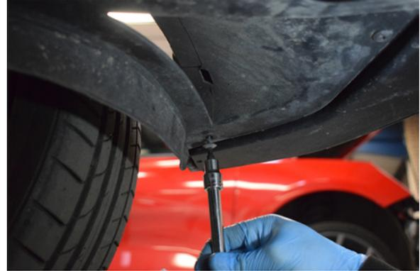
26. You can now undo and remove the outer screws under the front bumper.
