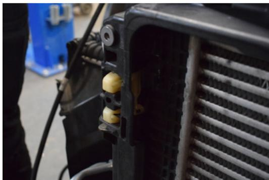
71. To remove the plastic frame in front of the intercooler, press the 2x plastic clips, you may need a helper to do this. (1 Clip per side)
