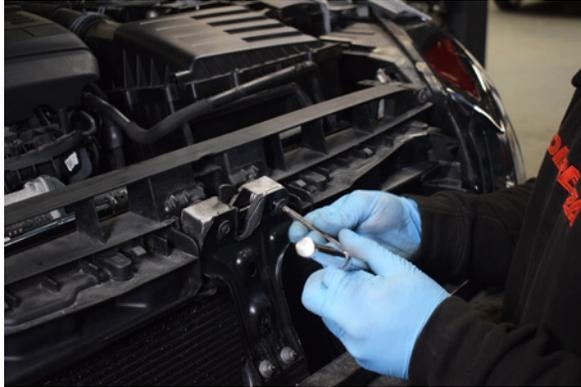
37. With the bumper removed you can remove the upper rad pack bracket.
