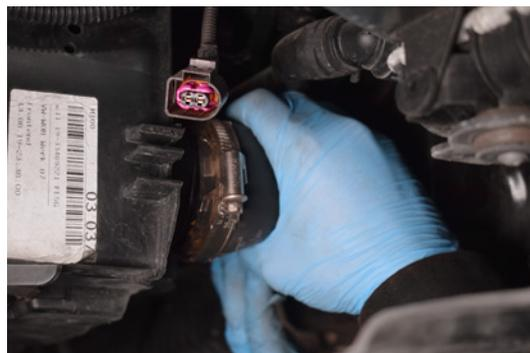
89. Push the OEM boost pipes over the MVT intercooler end tank outlet.
