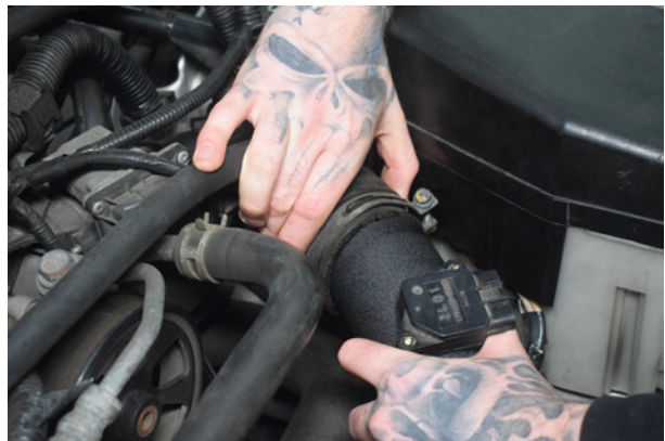
16. Insert into the OEM intake hose.
