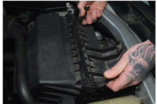
6. Pull back clips on the OEM airbox.
