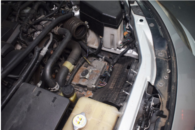
13. Pull the remaining section of the airbox and panel filter away from the studs.
