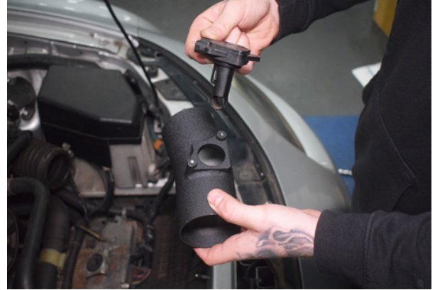
14. Insert the MAF sensor into the new aluminum intake pipe.
