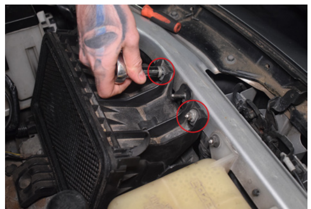
12. Remove 2x nuts securing the remaining section of the airbox to the car.
