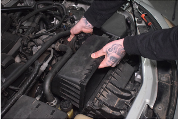
7. Remove the pictured section of the airbox.
