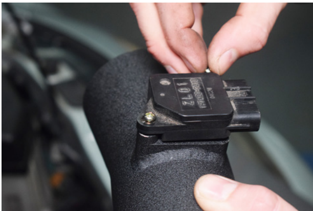
15. Secure using 2x screws supplied.
