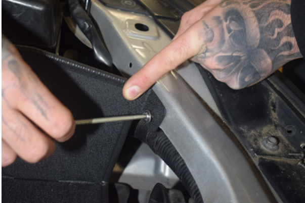
25. A screw can now be used to secure the airbox to the spire clip mounting position.
