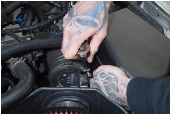
31. Fully secure the OEM intake pipe jubilee clip.
