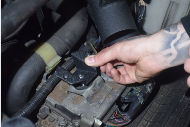
19. Place the mounting bracket into position.
