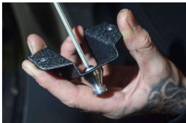
18. Install the bobbin onto the lower mounting bracket.
