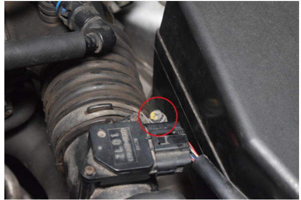
2. Undo 6mm Jubilee Clip on OEM intake pipe.
