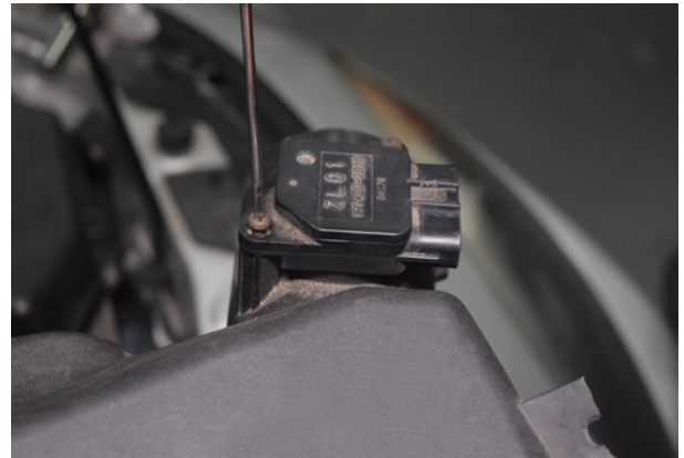
10. Remove 2x screws on the MAF sensor.
