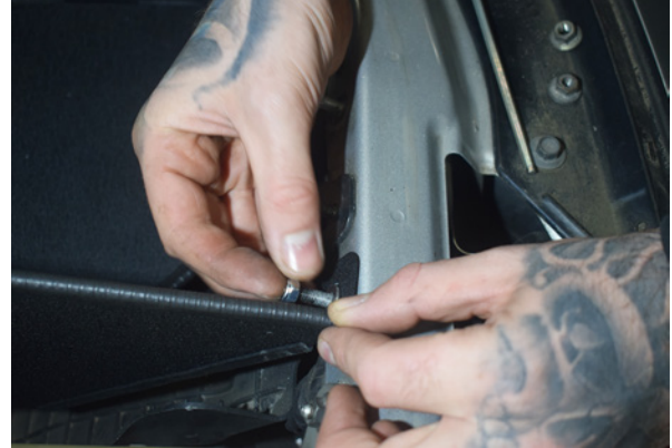
26. Install and tighten nut onto the mounting stud.
