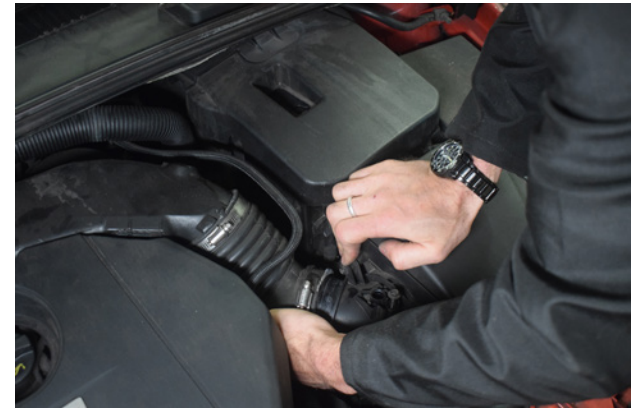
10. The intake pipe can now be removed.
