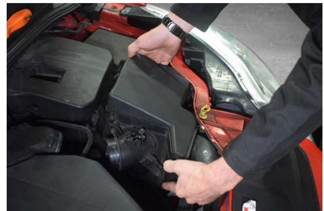
12. The factory airbox and filter can also be removed. This can be done by firmly lifting from underneath the box.
