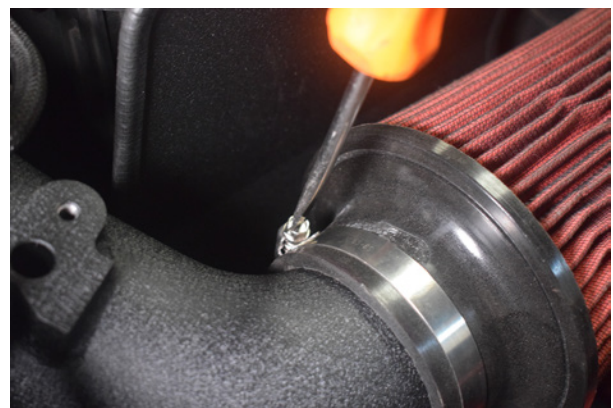
30. Tighten the jubilee clip to secure the Air Filter to the hard pipe.
