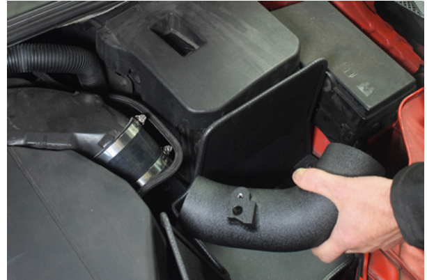
26. You can now install the aluminium intake pipe.
