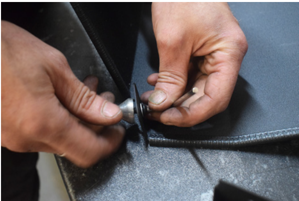
15. Before installing the Direnza shield, you will need to install all the bobbins included with the Kit.
