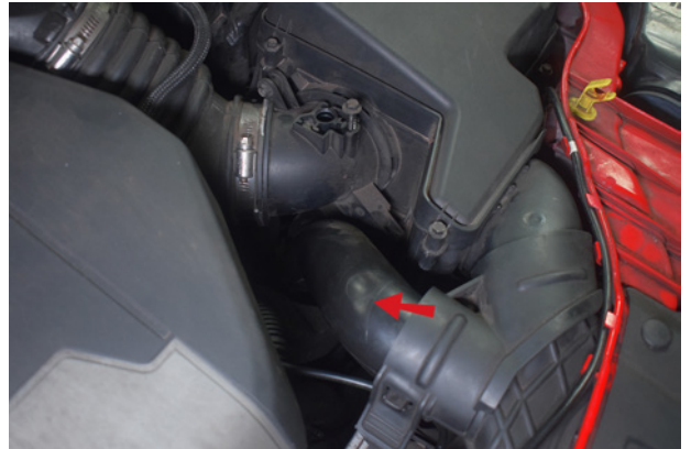
4. You can now remove the plastic intake pipe.
