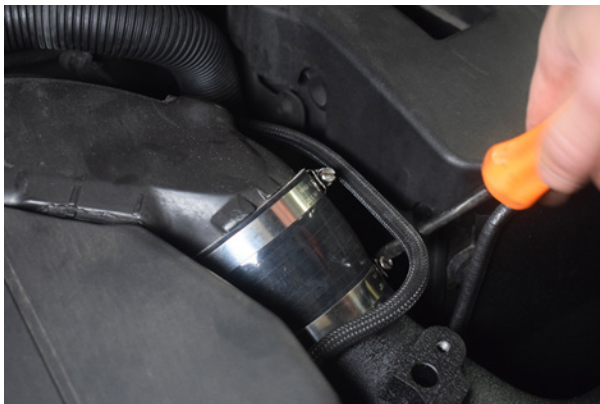
27. Tighten the jubilee clips to secure the silicone.
