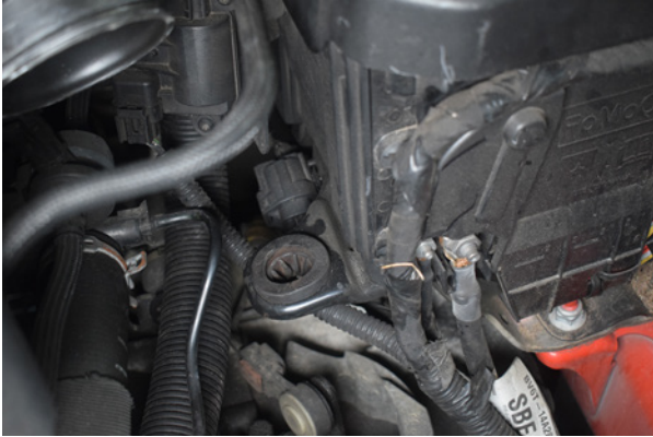
13. The Direnza heat shield fits into the factory mounting points.
