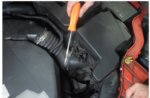
8. Undo the jubilee clips on the OEM intake hose.
