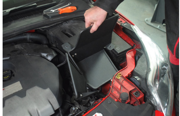
20. Place the Direnza heat shield in to position in the engine bay.
