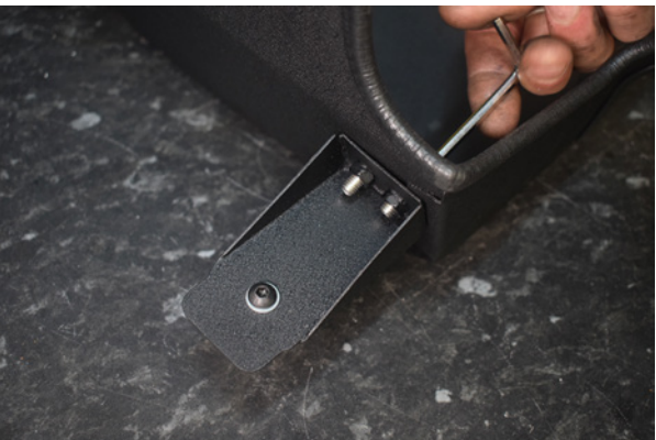
17. This bracket can then be fitted to the heat shield as pictured, using supplied hardware.
