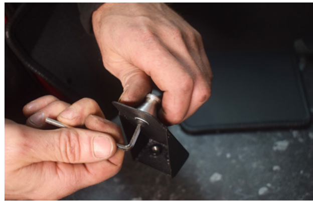
16. The second bobbin is fitted in this mounting bracket.
