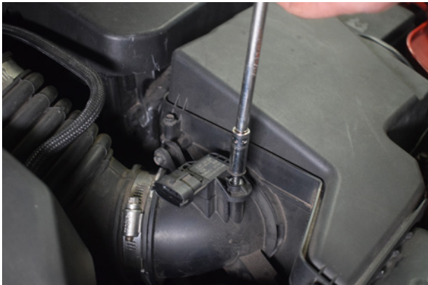
3. Remove the bolt on the MAF sensor using an 8mm socket.
