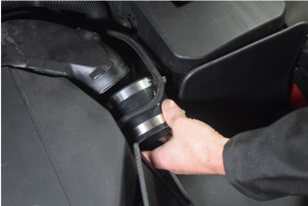
25. Install 2x jubilee clips around the supplied silicone joiner and fit onto OEM intake.
