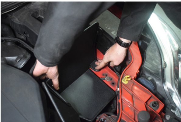
21. Secure by pushing down on the bobbin mounting points.
