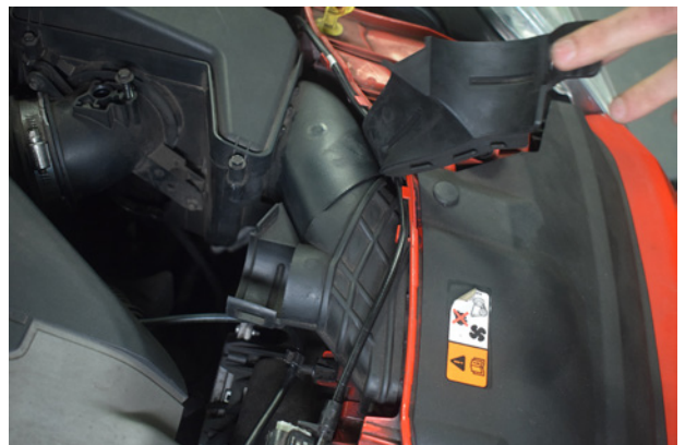
6. You can now remove the plastic slam panel scoop.
