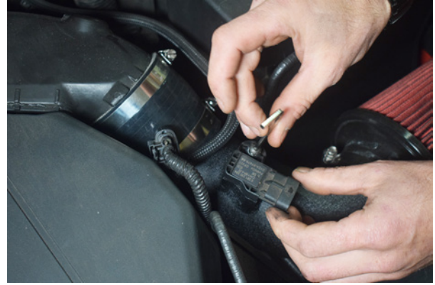
32. Using a 4mm allen key, install the MAF sensor.
