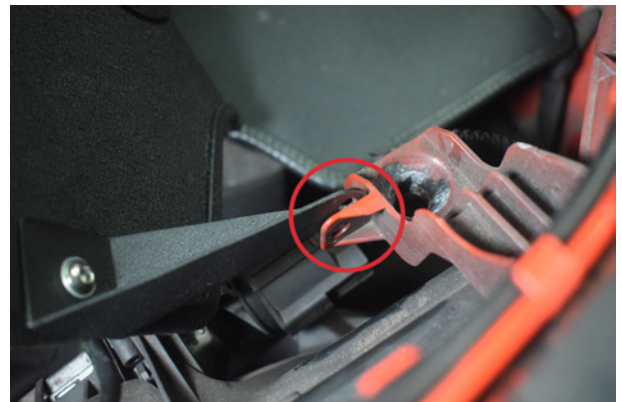
22. You will need install a nut, washer and bolt to secure this part of the mounting bracket to the car.
