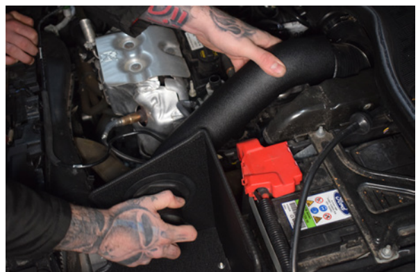
30. You can now install the hardpipe, insert through the Airbox and then into the silicone joiner.
