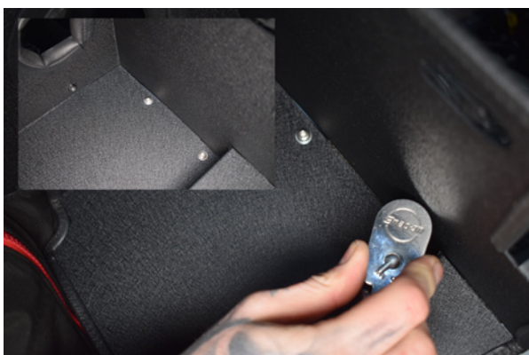
17. Hold the bobbins and tighten from the top.
