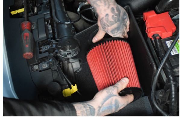
32. Install the Air Filter and jubilee clip.
