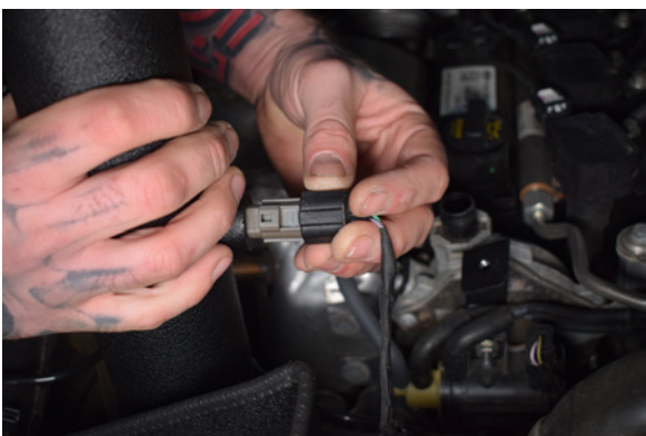
29. Before installing the hard pipe remember to plug in the MAF sensor as this sits underneath.
