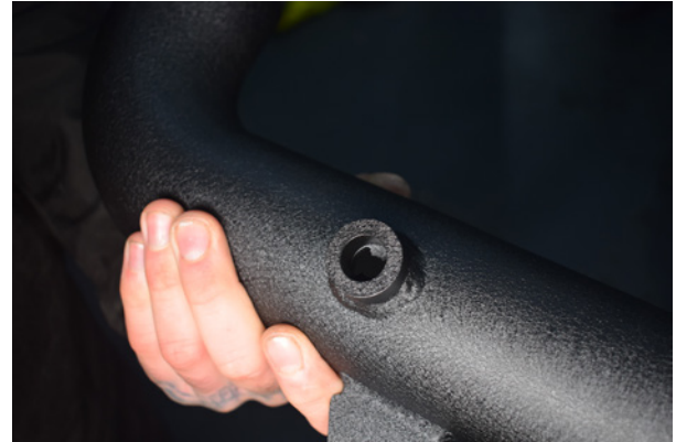
14. Insert this sensor into the Direnza hard pipe.
