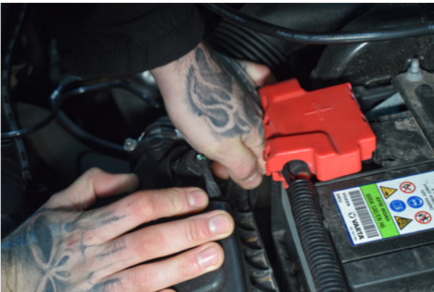
3. Remove clip from underneath the intake pipe.
