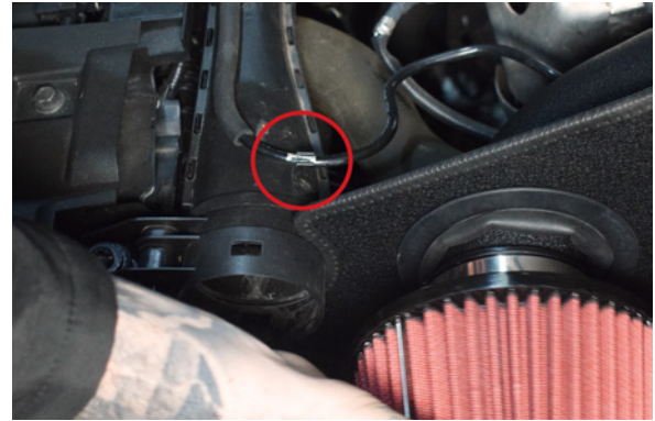
38. Re fit pipe into the clip on the air snorkel.
