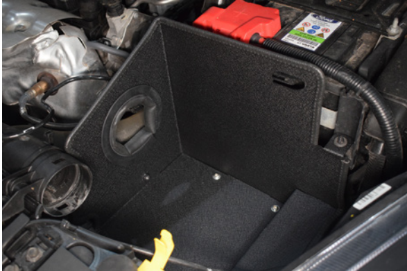
19. Install the Direnza box into position.
