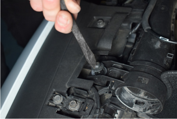
31. Re-secure the slam panel snorkel.
