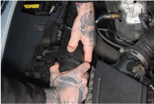
7. Separate the snorkel from the airbox.
