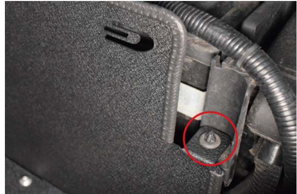
20. Ensure the rubber O ring is properly inserted into the box and mounting point.
