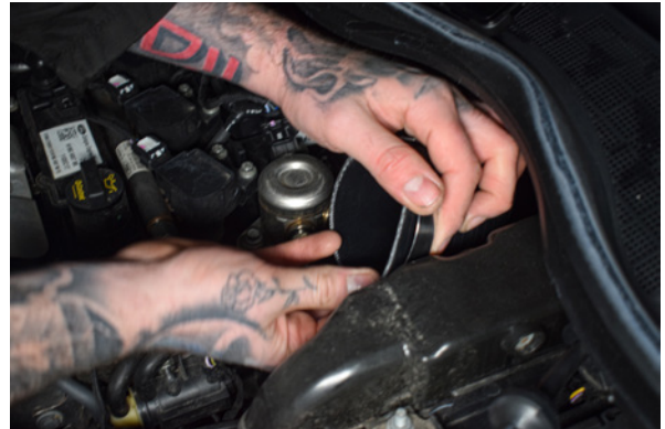
28. Install second jubilee clip on the 90° silicone.
