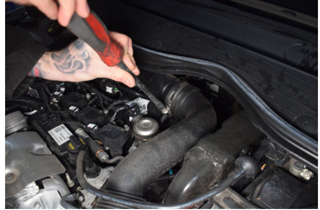
2. Undo jubilee clip connecting the induction hose to the throttle body..
