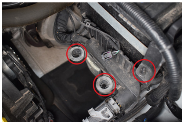
11. The Direnza box sits on the factory mounting points.
