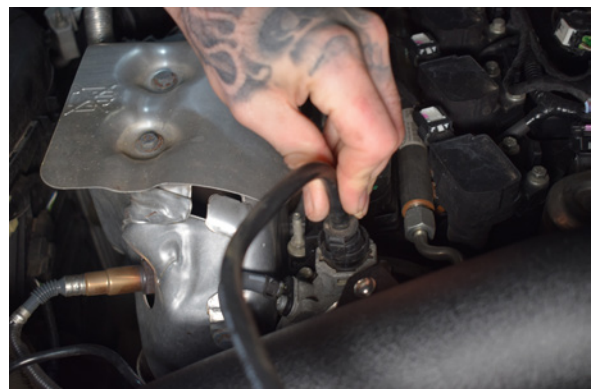
36. Re-install the vacuum pump line.
