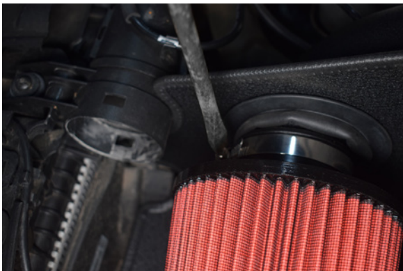
39. Fully secure the Air filter to the hard pipe by tightening the jubilee lip.
