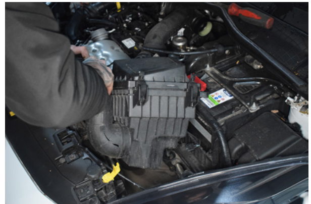
10. The airbox assembly can now be removed.
