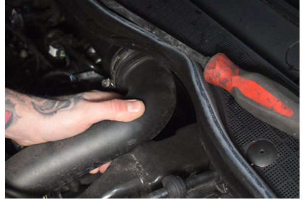
8. Remove intake pipe from the throttle body.
