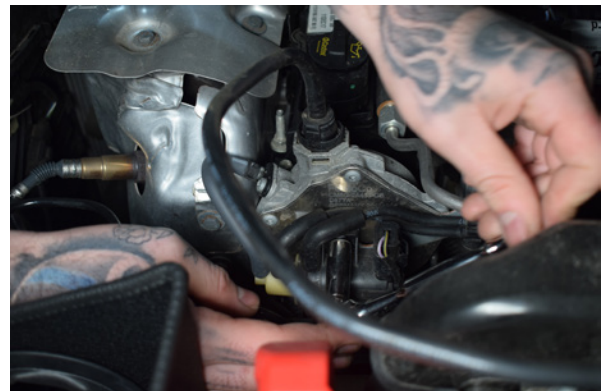
22. Remove upper nut on the vacuum pump to allow the Direnza support bracket to be mounted behind.
