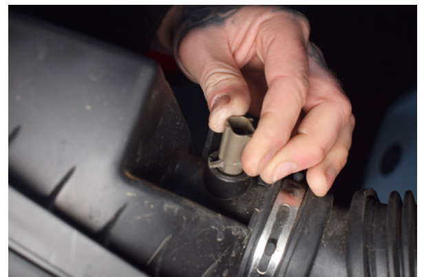
12. Remove sensor from factory airbox.
