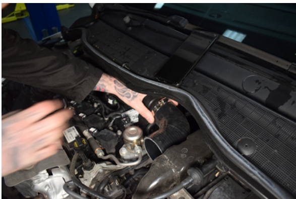
21. Install the 90° silicone and nip tight with jubilee clip to allow for some slight movement.
