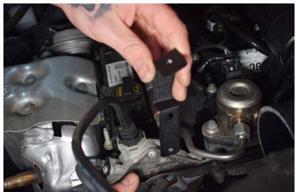
24. The Direnza support bracket sits behind the vacuum pump in this orientation.
