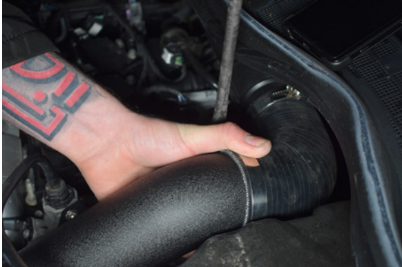
37. Secure the hardpipe in the 90° silicone by tightening the jubilee clip.
