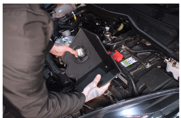
18. You can also fit the edging trim around the box and inside the exit hole for the hardpipe before installing.
