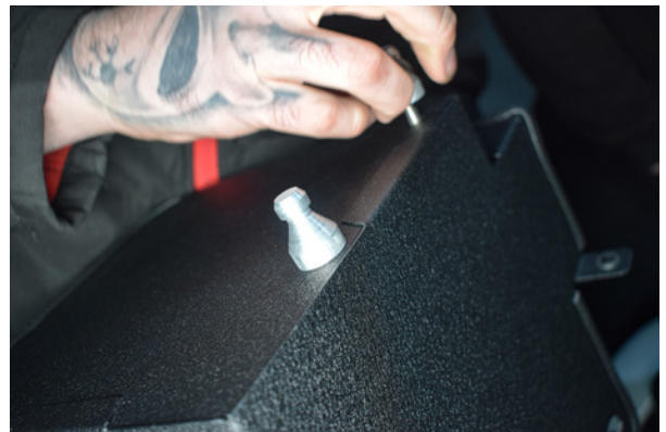
16. The mounting bobbins can then be installed by threading them onto the screws.
