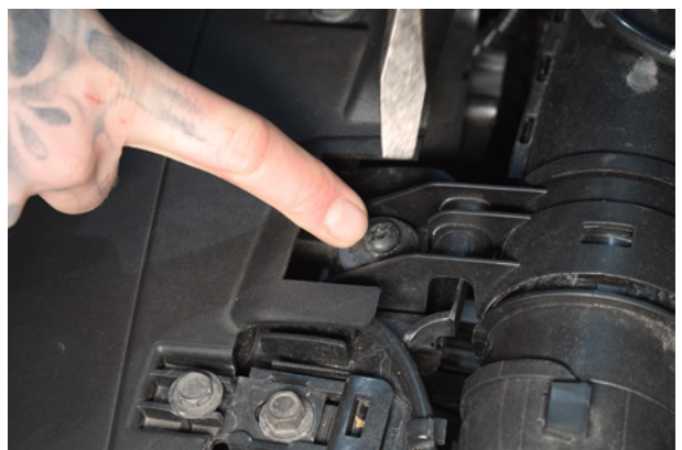
6. Undo screw securing the air snorkel to the slam panel, this allows some movement to remove the factory airbox.
