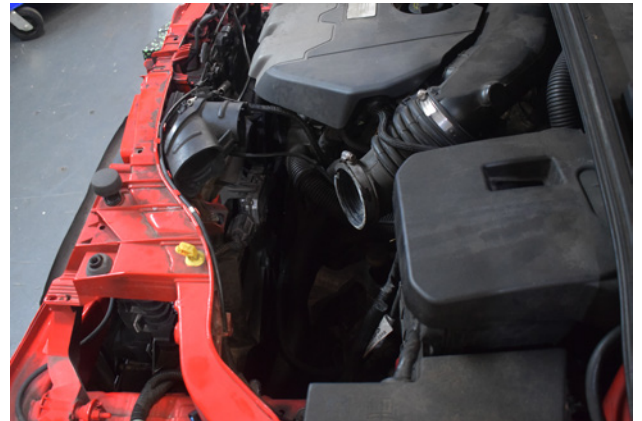
46. You can now remove the rear section of the air ducting
