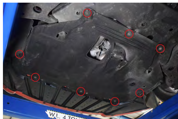
65. Fit engine undertray and secure using 8x screws.
