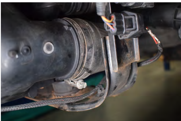
29. Undo jubilee clip securing the intercooler to the hot side pipework.
