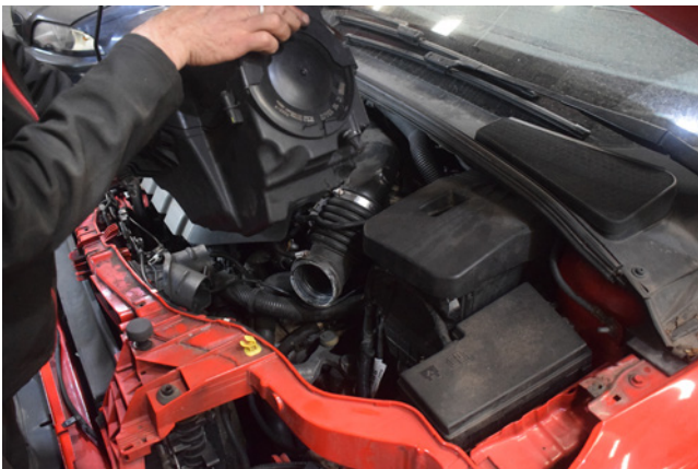
45. You are now able to remove the Air Box as a complete unit.
