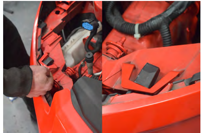
26. Lift bumper release tabs.
