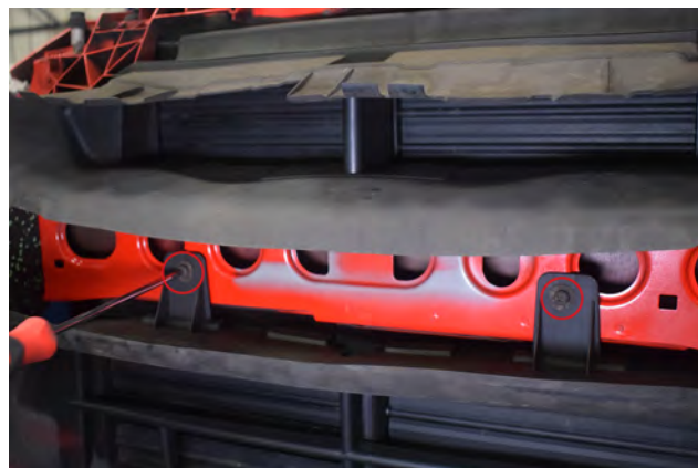
34. Undo 2x T30 screws and remove large ducting panel.
