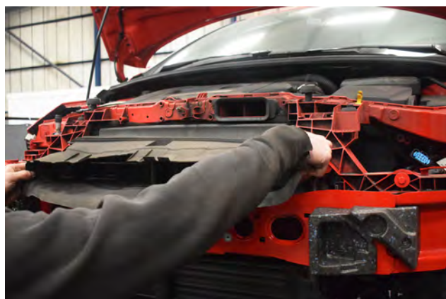
35. The top duct can be removed with a gentle pull.
