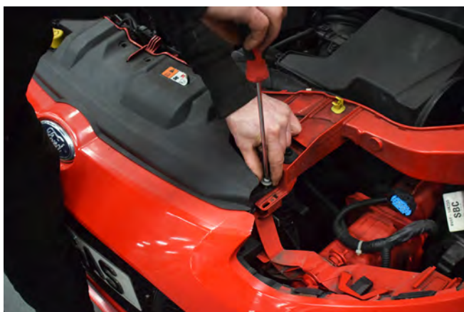
9 Remove the 2x T30 screws at either end of the slam panel cover.
