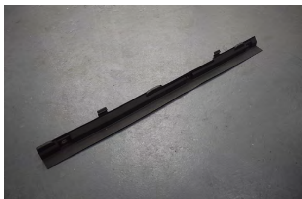
66. Fit plastic diffuser lip using 3x Torx.
