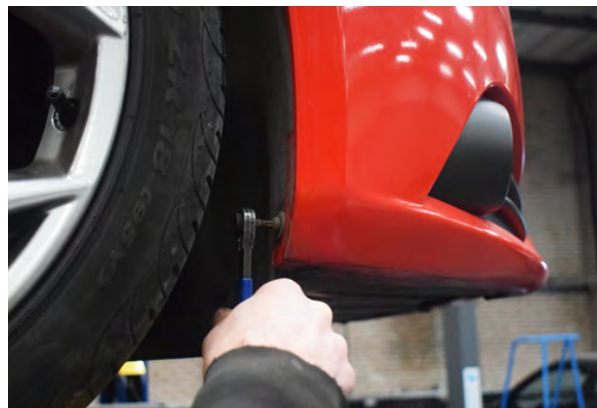
62. Install lower inner arch T30 screw.
