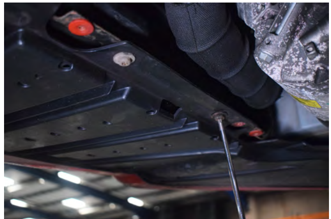
18. Remove 3x T30 screws from the back section of the bumper under tray.
