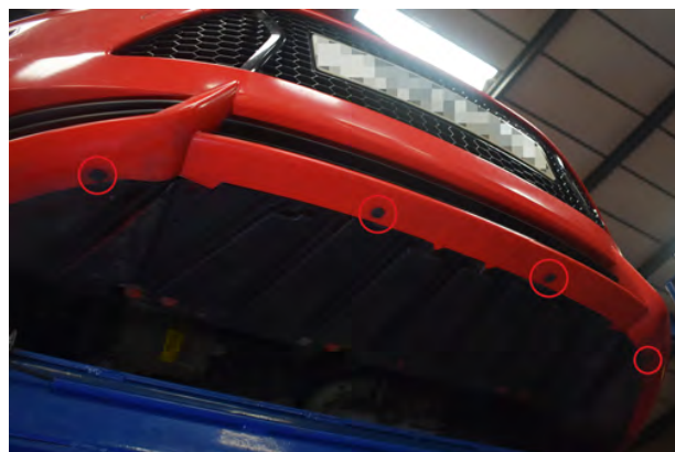
64. Push all plastic trim clips into the underside of the front bumper.
