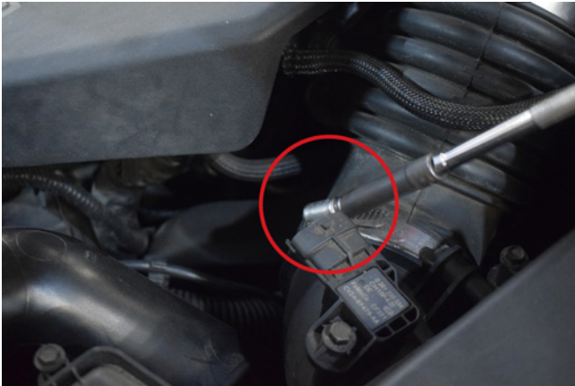
43. Undo jubilee clip located near to the MAF sensor.
