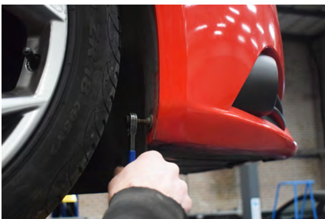
17. Remove 1x T30 from the inner wheel arch. This needs to be done both sides.
