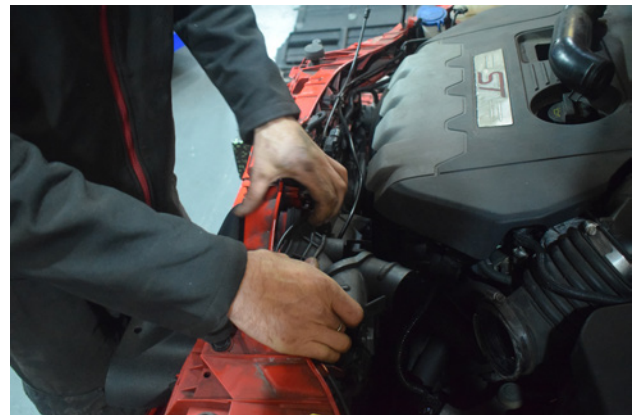
54. You can now re-install the OEM ducting behind the scoop.
