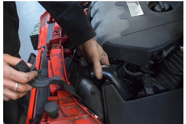
42. You can now begin removing the Airbox.
