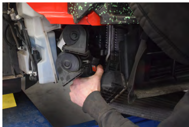
32. Lift and tilt the intercooler to remove from locating tabs and release from pipework.
