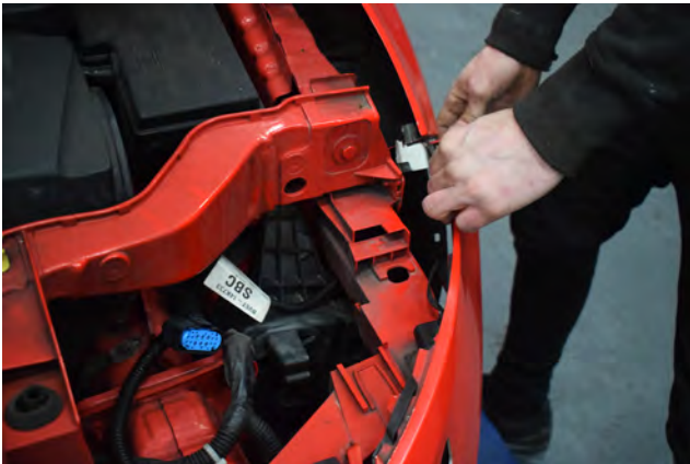
25. Lift and pull both edges of the front bumper to release from position.
