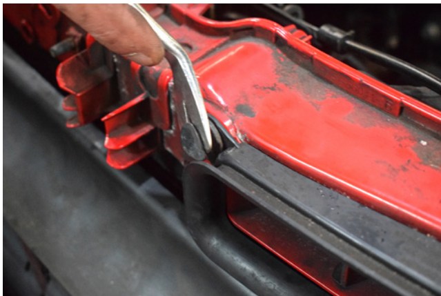
39. Remove the small OEM air duct by removing the 2x plastic trim clips.
