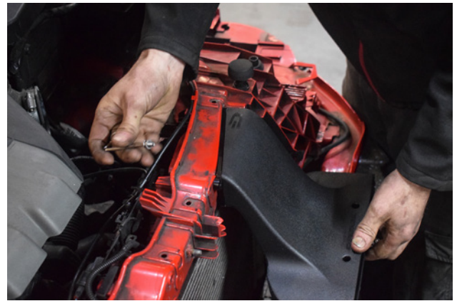
50. Using 2x bolts and washers secure the scoop to the front panel.
