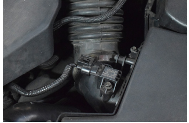
58. Plug the MAF sensor back in.
