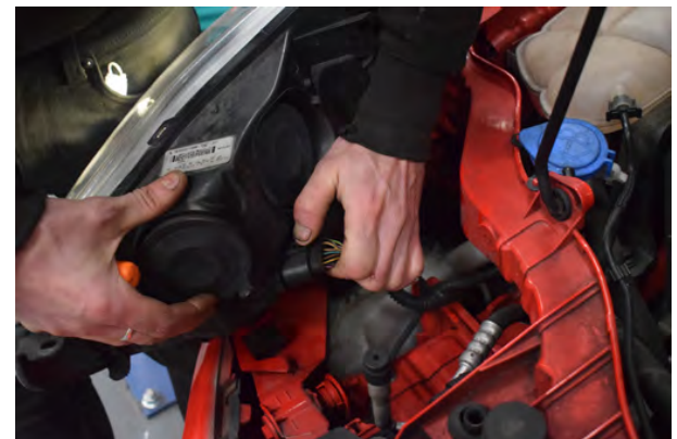
70. Re-connect headlights to plugs.
