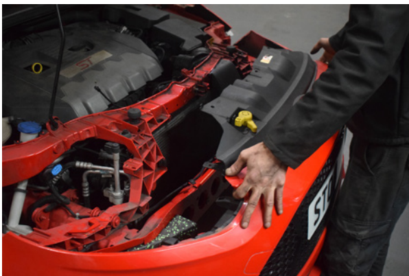
59. Re-fit the front bumper and push the sides into position. Re-install all associated hardware. REMEMBER to plug in front bumper wiring loom.
