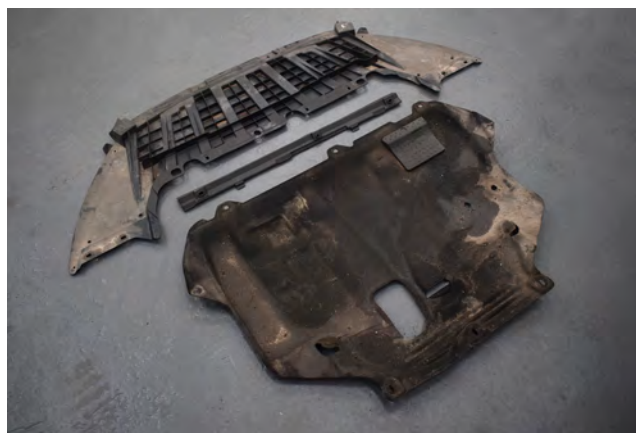
20. Pictured, all the undertray items you have just removed from the car.
