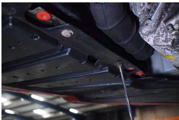
61. Install front bumper undertray and secure using original hardware.
