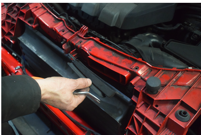
41. Remove the duct.
