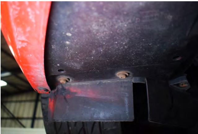
15. There are also 4x T30 screws (2 per side) on the outer edge of the front bumper under tray.
