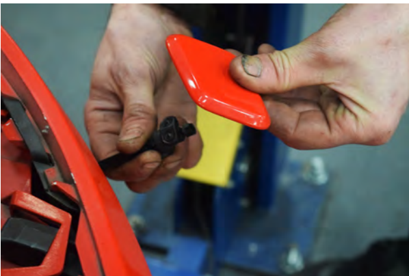
69. Install washer jet covers.
