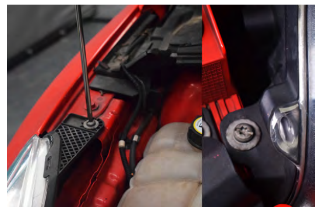
72. Secure the headlights using 2x T30 screws. Do this for both sides.
