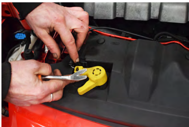
7. Remove the bonnet safety catch.
