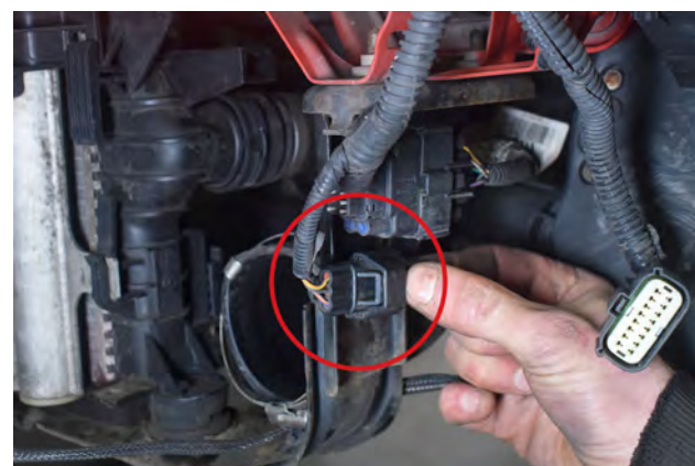
36. Unplug flap control panel.
