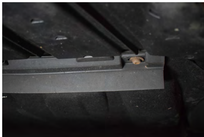
10. Remove the plastic diffuser lip from underneath the car by undoing 3x torx bits.
