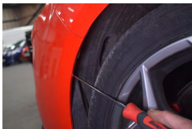
22. Remove T30 screw (1 per side) from higher up in the inner wheel arch.
