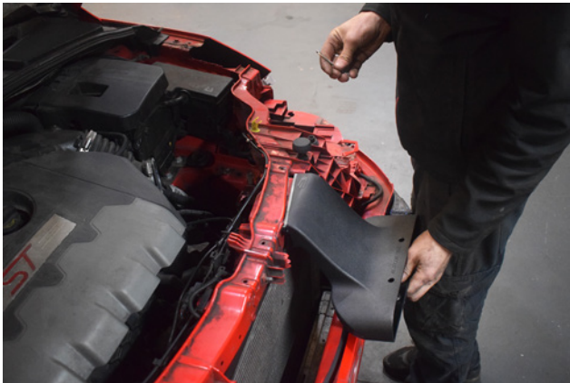
49. Place the Scoop into position onto the front of the car.
