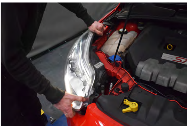
71. Install the headlights, once seated in the correct position.
