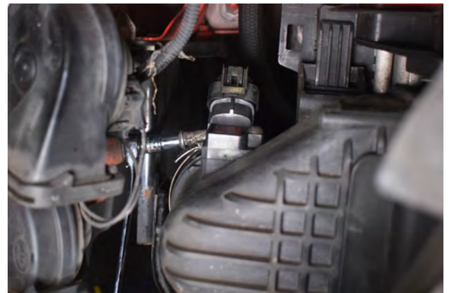
28. Undo jubilee clip securing the intercooler to the hot side pipework.
