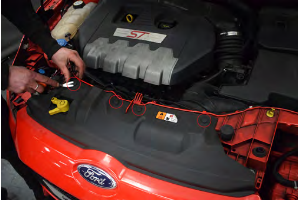
67. Install 4x plastic trim pieces on the slam panel and 2x T30 screws at each end.
