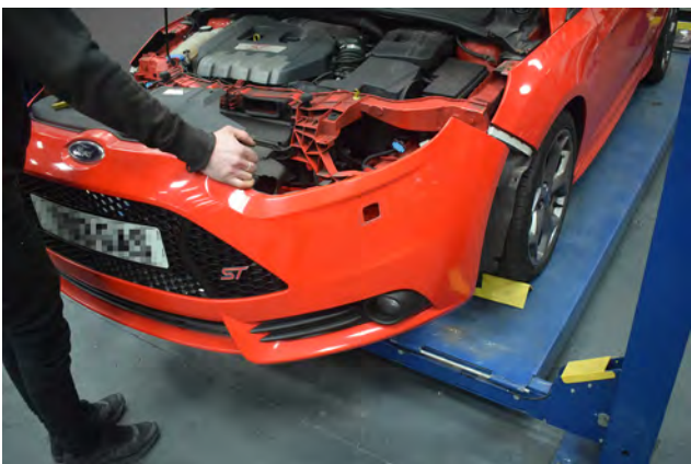
27. The front bumper can now be removed. Store in a safe location.
