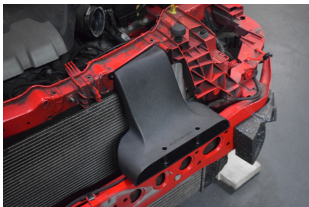
53. The Vortex Scoop is now installed
