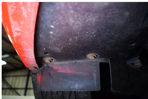
63. Install 4x T30 screws on the other edge of front bumper undertray (2 per side).
