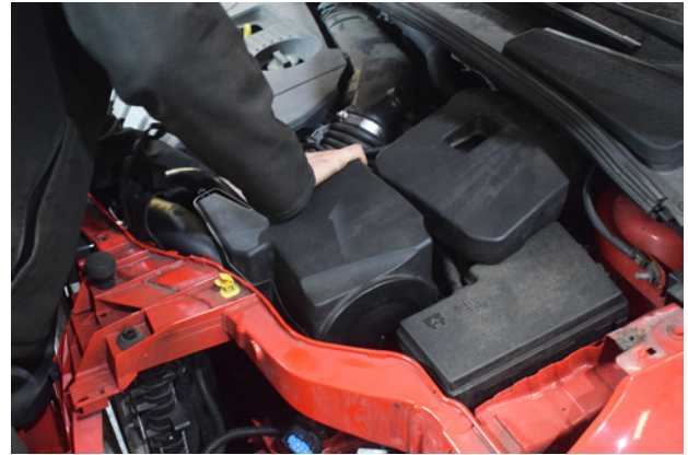
56. Place the Air Box back into position.
