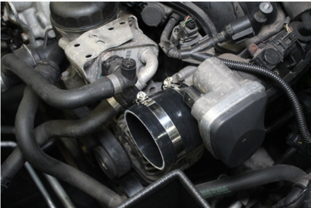
21. Fit silicone joiner and 2x jubilee clips onto the throttle body.
