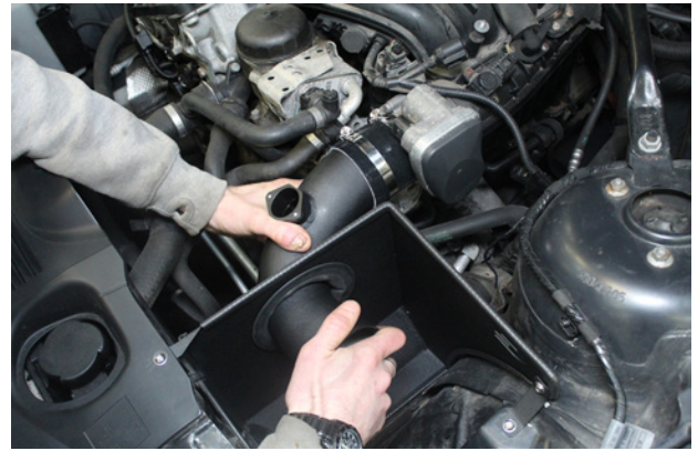
22. Work the new Direnza intake pipe into position.
