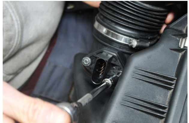
26. Remove the MAF from the OEM intake pipe.
