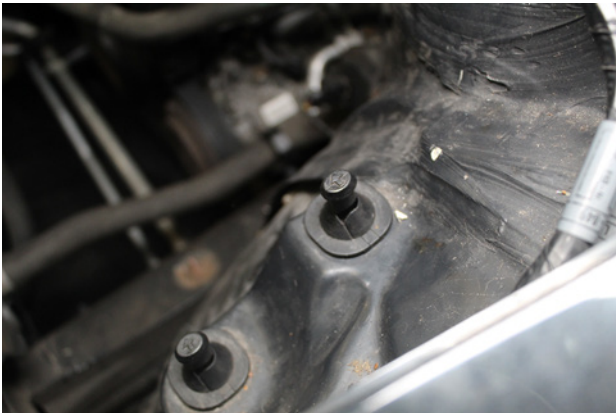
9. Locate the higher of the two plastic bobbins on the inner wing.
