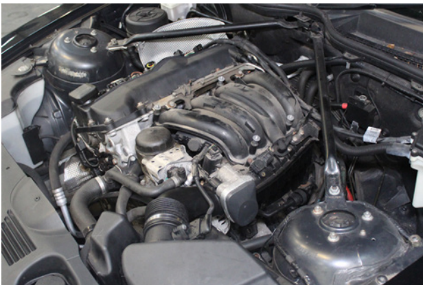
3. Pull off the engine cover.
