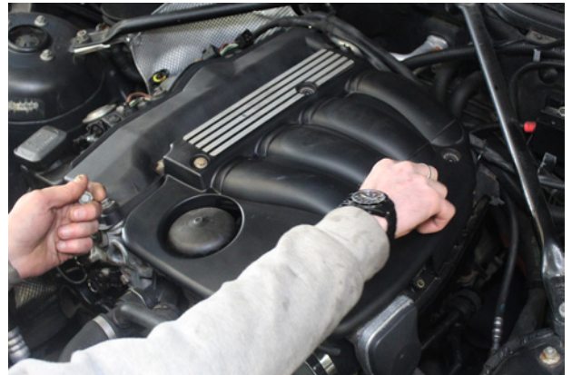
30. Re-fit engine cover using 4x 10mm nuts.
