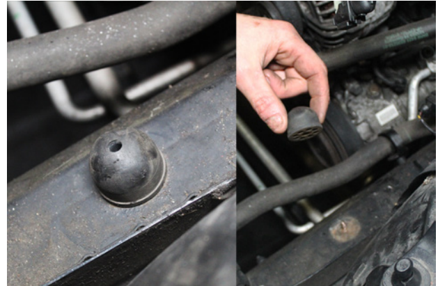
8. Remove rubber bobbin, this just pulls off.
