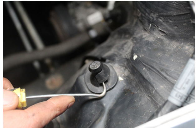
10. Remove this plastic bobbin using a pick and twisting 90 degrees.
