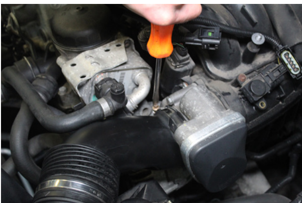
5. Undo jubilee clip on throttle body.
