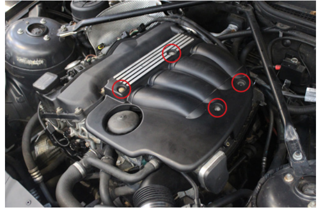
2. Undo 4x 10mm nuts on the plastic engine cover
