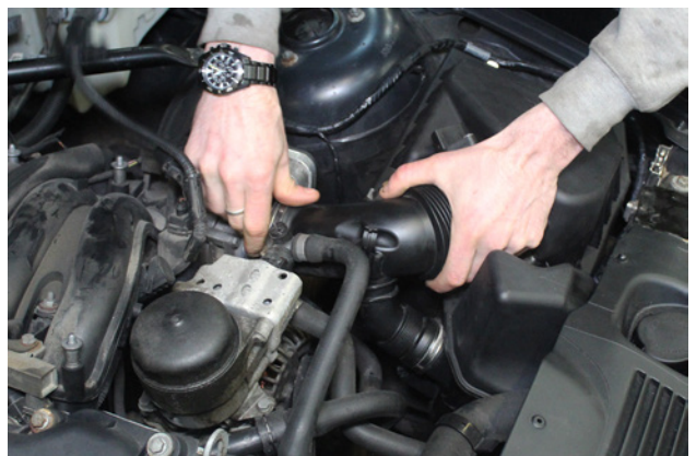
6. Pull air intake pipe away from the throttle body.
