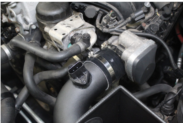
27. Place the MAF into the Direnza intake pipe.
