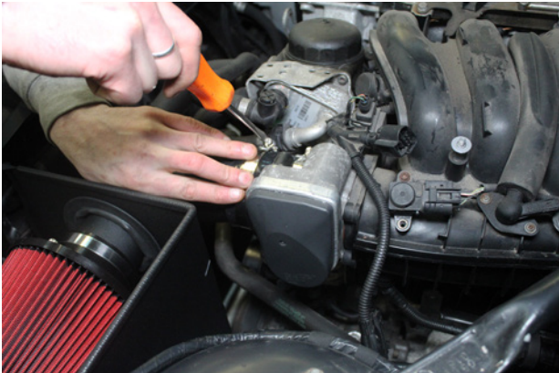
25. You can now fully tighten all jubilee clips to secure the filter and intake pipe.
