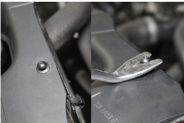
11. Locate and remove the further most (Passenger side) trim clip on the plastic slam panel.
