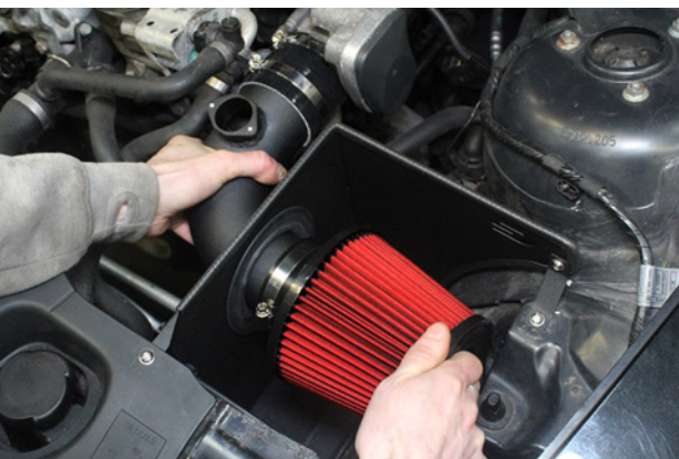
23. Fit the air filter onto the end of the intake pipe inside the airbox.
