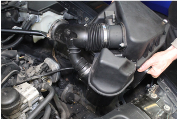
7. Pull out the airbox out, this can require a little force.
