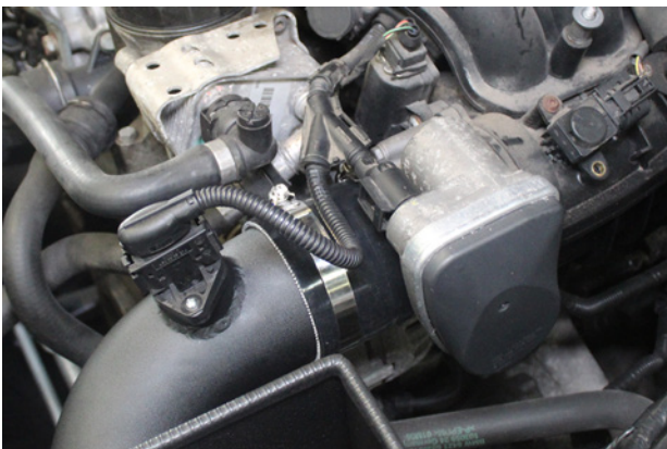
29. Reconnect MAF and throttle body plugs.
