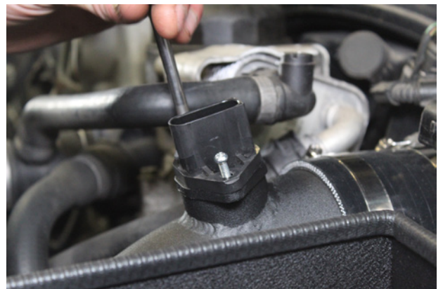
28. Secure the MAF using supplied screws.
