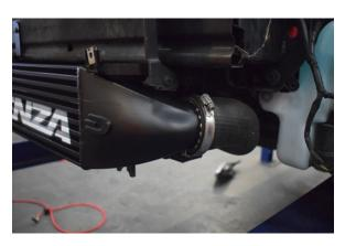
42. Install the intercooler hoses onto the MVT intercooler end tanks.
