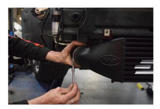
43. Tighten the OEM jubilee clips with 7mm socket.
