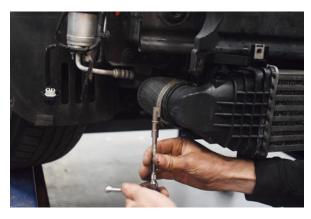
28. Undo 2x jubilee clips on the OEM intercooler using 7mm socket.
