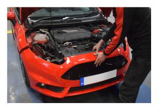
47. Lift the front bumper back into position.
