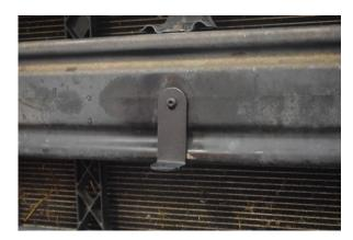
37. Install the bracket onto the crash bar using the 4mm allen bolt, nut and washer.
