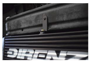
38. Lift the MVT intercooler into position and secure to the mounting bracket using the supplied 13mm bolt.
