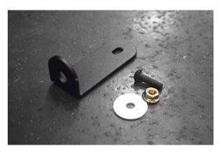
36. Locate the supplied intercooler bracket in the MVT kit.
