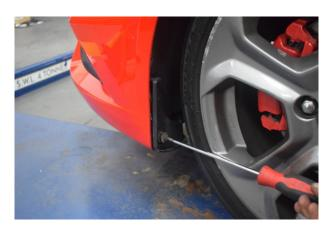
9. To take off the bumper start by removing 4x screws located along the leading edge of the arch liner.
