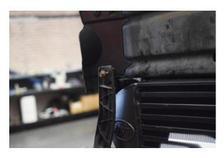
44. Re insert lower shroud trim and install 5x 8mm bolts.
