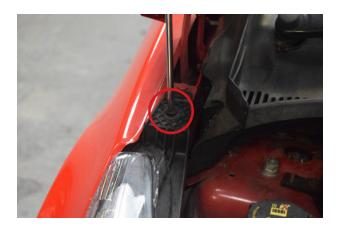
2. Remove 2X T30 to remove the headlight.
