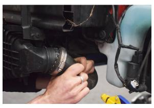
30. The OEM boost hoses can now be pulled off the intercooler.
