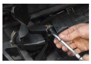
21. You can now remove the intercooler shroud by removing 5x 8mm bolts. 2x at the top and 3x located underneath.
