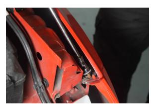
51. Install 3x 10mm inner wing bolts and repeat on the other side.
