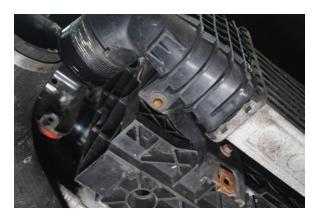
32. From underneath, remove 2x 8mm bolts on the lower intercooler mounting points.
