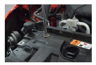
49. Install 2x T30 screws into slam panel.
