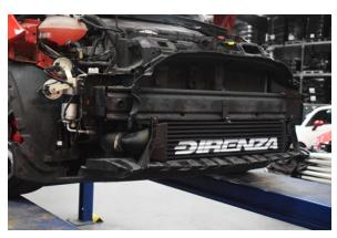
46. The intercooler is now installed and the front of the car can now be rebuilt.
