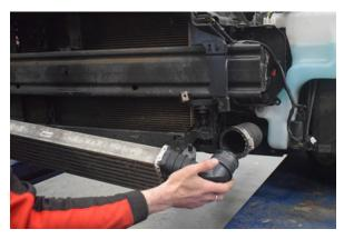
34. The intercooler can now be removed from the car.
