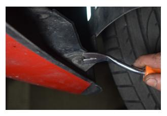
13. Remove plastic clip from under front bumper, one per side.
