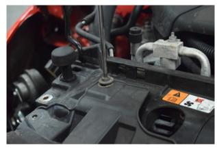
16. Remove 2x T30 screws also located on the slam panel.
