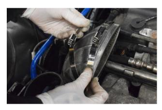
16. Slide the clips over the hot side hard pipe.
