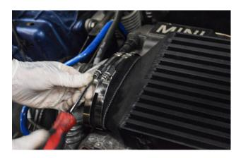
18. Tighten supplied jubilee clips to secure the intercooler.
