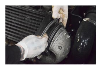
10. With the screws removed, the C clamps can be removed or left loose until the intercooler is out.
