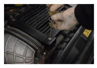
2. Remove 4X T30 screws securing the intercooler cover.
