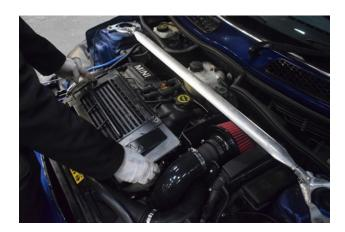
4. Once all four T30's have been removed you can lift off the cover.
