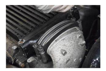
7. You can now remove the 4x T30 screws on the factory 'C' clamps.
