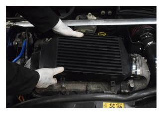
13. The intercooler needs to be pushed into the cold side joiner/hardpipe first.
