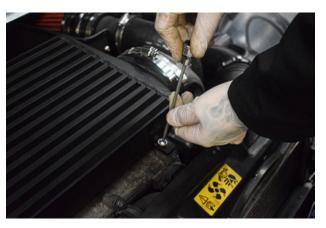
14. Use supplied hardware to secure the intercooler brackets.
