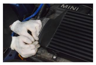
16. Manipulate the intercooler in to position on the hot side.
