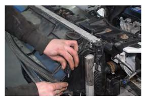
117. Install top ducting with clips.
