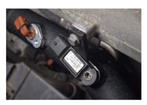
67. Fit the pressure senor into the cold side hard pipe.
