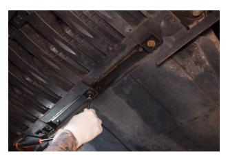
1. Remove 7x 10mm bolts from the engine under tray.
