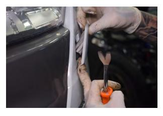
10. Remove the washer jet by pulling out the mechanism and rolling off plastic cover.
