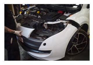
16. Lift and pull the bumper to release.
