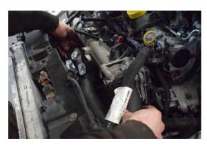
61. Install the first section of the cold side hard pipe onto the throttle body.
