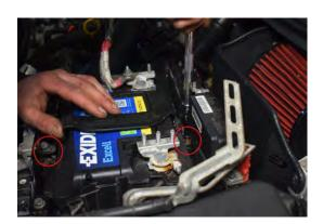
112. Secure the battery with 2x 8mm bolts and battery bracket.
