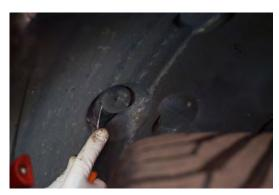
131. Install 3x push clips under the wheel arch, repeat on both sides.
