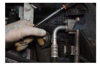
35. Remove 10mm bolt from the cold side boost pipe support bracket.
