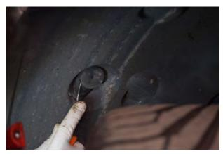
7. Remove 3x push clips under the wheel arch, repeat on both sides.
