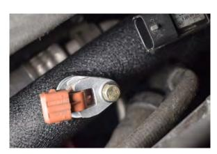
66. Fit the temp sensor and supplied support bracket with supplied 10mm screw.
