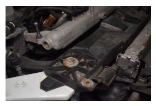
52. Undo 2x 13 bolts on the plastic slam panel.
