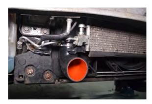
91. Place the large 90° silicone and jubilee clip facing forward onto the end of the cold side hard pipe.
