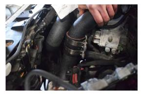
83. Slot the two pipes together with the silicone joiner and secure with 2x jubilee clips.
