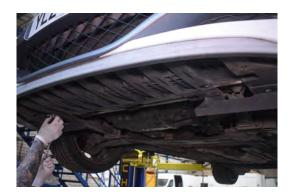
135. Install 4x 10mm bolts from bumper under tray.
