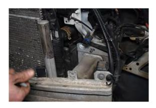
86. Secure using 6x 16mm bolts, (three per side).
