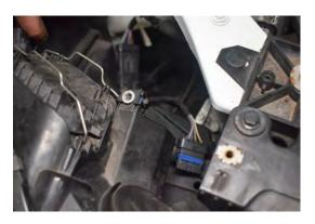
122. Re-install 2x headlight connections and place into position.
