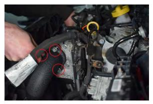
62. Install 3x 10mm bolt securing the new Direnza hard pipe to the throttle body.
