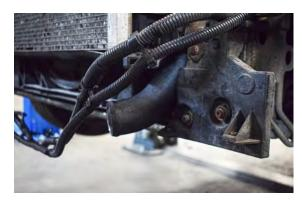
82. Feed the second hard pipe into position from the bottom upwards.
