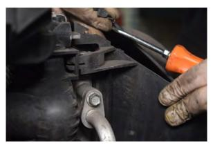
54. Use screwdriver to push clips holding the front cowling.
