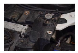
19. Remove 3x 10mm screws from the from the headlight holder.
