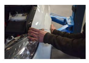
127. Push in the sides of the bumper once fitted in position.
