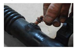
64. Remove sensor from the OEM pipe.
