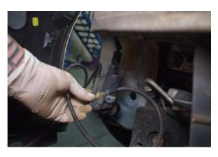
18. Unplug washer jet pump and move bumper to a safe place.
