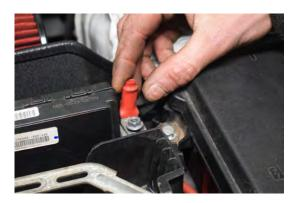
110. Fix with further 2x 10mm bolts ensuring battery terminal is attached.
