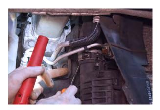
36. Undo the clip on the cold side boost pipe, releasing the intercooler.
