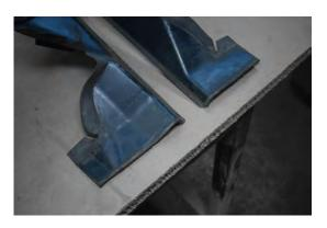
115. The side ducting requires a small amount of trimming to fit around the larger intercooler.
