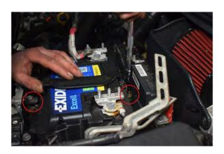
27. Remove 2x 8mm bolts securing battery holder bracket.
