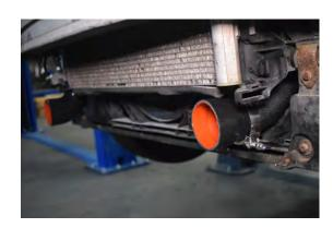
94. Place 2x clips clips onto the end of the hardpipes.
