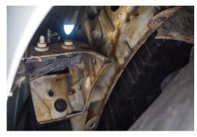
129. Install 3x 10mm screws under the liner and 1x T25 do this on both sides.
