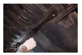
136. Install 7x 10mm bolts from the engine under tray.
