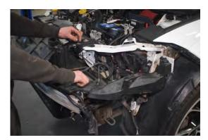
119. Install the headlight holder and secure with 3x 10mm bolts. Do this on both sides.
