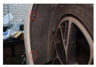
6. Under the wheel arch, remove 2x T20 torx, do this on both sides.
