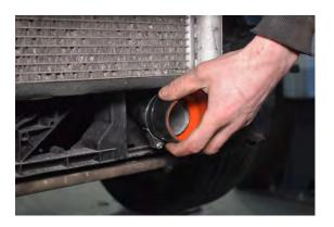
92. Secure the final silicone onto the end of the hot side hard pipe.
