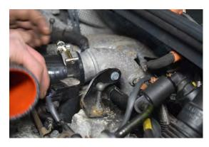
77. Place into position on the turbo outlet.
