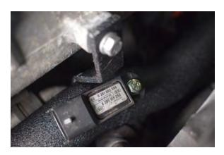
68. Secure sensor with supplied 10mm screw.
