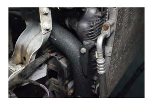
73. Secure 2nd support bracket with supplied 10mm bolt.
