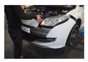
126. You can now begin re-fitting your front bumper remembering to reconnect the washer jet pump and wiring harness.
