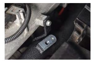
63. Fit 10mm bolt on the front upper support bracket.
