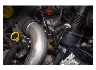
42. Remove 2nd 10mm on the boost pipe bracket.
