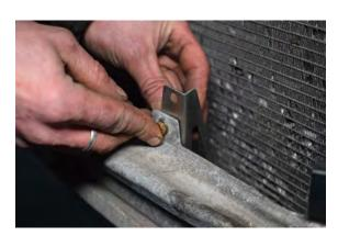
89. Secure the intercooler brackets into position on the lower of the two mounting holes with supplied nuts and bolts.
