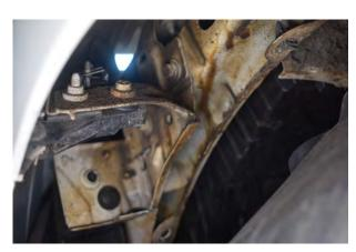
9. Remove 3x 10mm screws under the liner and 1x T25, do this on both sides.
