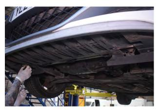
3. Remove 4x 10mm bolts from bumper under tray.
