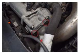
46. Remove 3x 10mm bolts on the throttle body inlet pipe.
