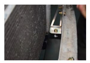
98. Secure the MVT intercooler to the support brackets with supplied bolts.
