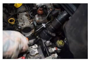
50. Undo the jubilee securing the cold side boost pipe to the sound enhancer unit.
