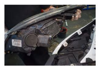
13. Lift and remove headlight, remembering to unplug all connections.
