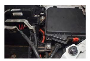
109. Locate fuse box pins /brackets on battery tray and secure with 2x 10mm bolts.
