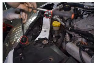
11. Remove 2x 10mm bolts and lift metal clip securing the headlight.
