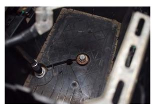
33. Undo 3x 13 bolts holding the battery tray to the car.
