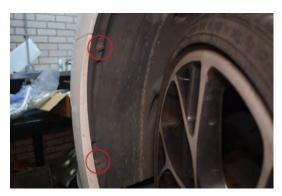
132. Under the wheel arch, install 2x T20 torx, do this on both sides.
