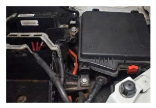
30. Remove 2x 10mm bolts on the cover and remove.
