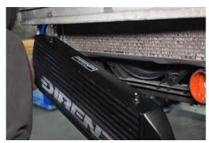
95. Place intercooler into position in the silicone joiners.
