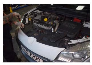
4. Remove 6x T20 torx from the top edge of the front bumper/slam panel.
