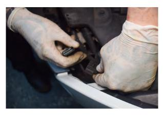
17. Unplug the wiring harness located on the passenger side of the vehicle (RHD drive models).
