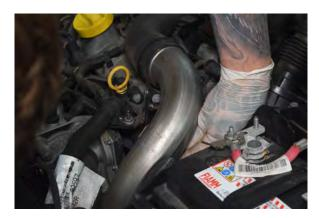
43. The 3rd 10mm to remove is hidden under the boost pipe.
