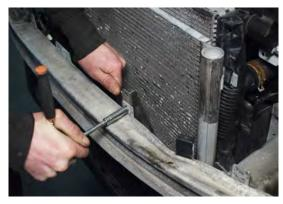
100. You can now tighten all the 10mm bolts securing the intercooler and brackets.
