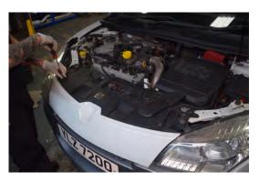
134. Install 6x T20 torx from the top edge of the front bumper /slam panel.
