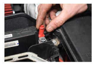
29. Remove 2x 10mm bolts and battery terminal.
