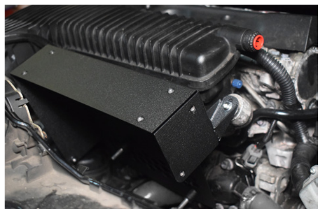
24. Line up the bobbins and push the bracket into position.
