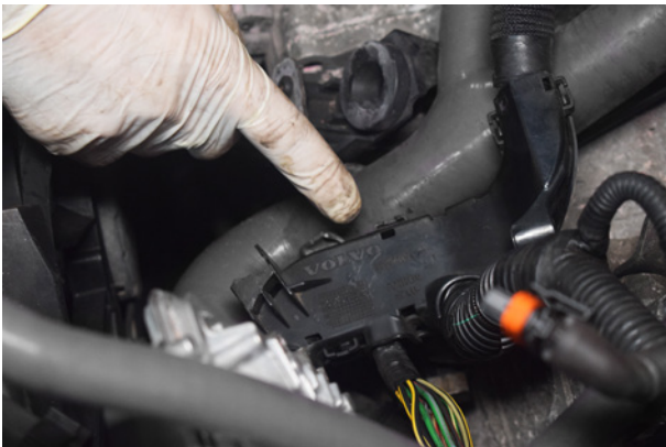
21. Remove wiring loom trim. This comes off in two pieces.
