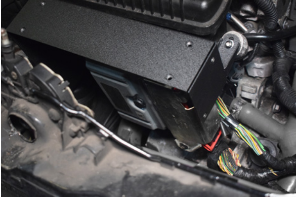
25. Install ECU onto mounting pegs.
