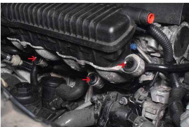
23. This bracket pushes into factory fixing points.
