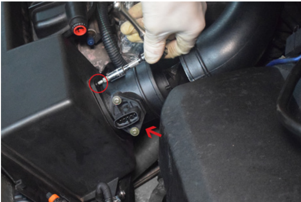
13. Undo 2x T20 and remove MAF.
