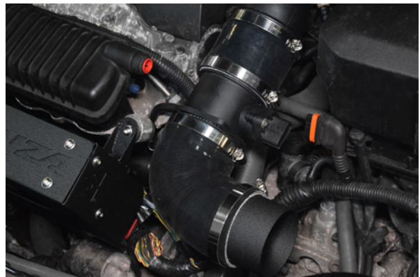
40. If required, rotate the MAF into the correct position.
