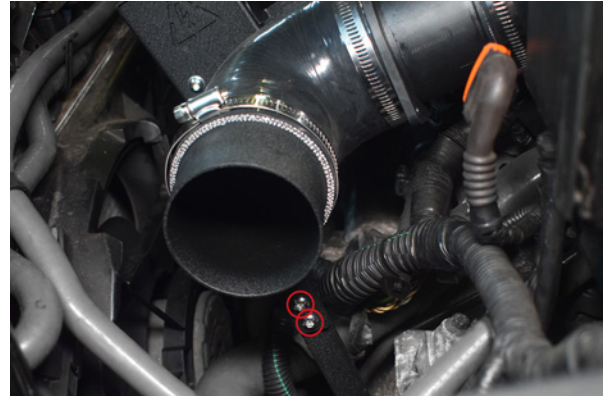
38. Line up bracket holes and secure together using supplied hardware.
