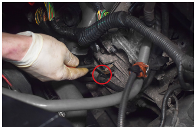
30. Use trim tool to remove wiring from clip/bracket.
