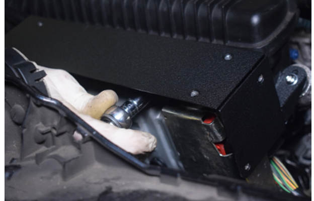
26. Secure ECU with 3x 10mm nuts (supplied).
