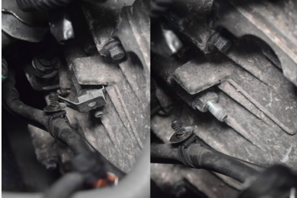
31. Use 13mm socket to remove bracket.
