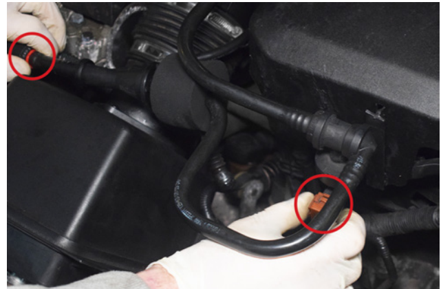
8. Remove Vacuum pipe and plug.
