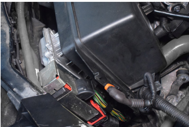
17. We will have to unscrew the ECU on the car by removing 4x T20 screws.
