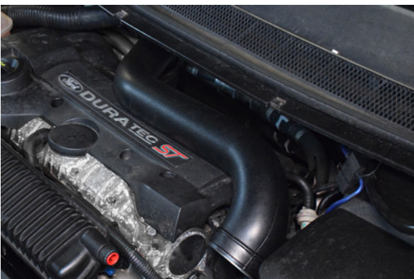
29. You can now tighten the 3x 10mm bolts on the crossover pipe.
