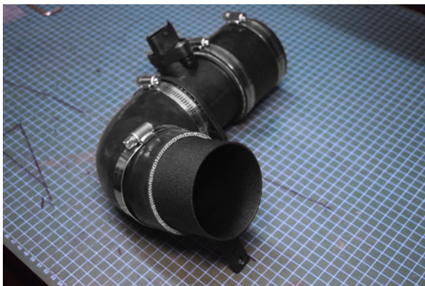
35. Install 90 degree silicone & aluminum adapter pipe with bracket.
