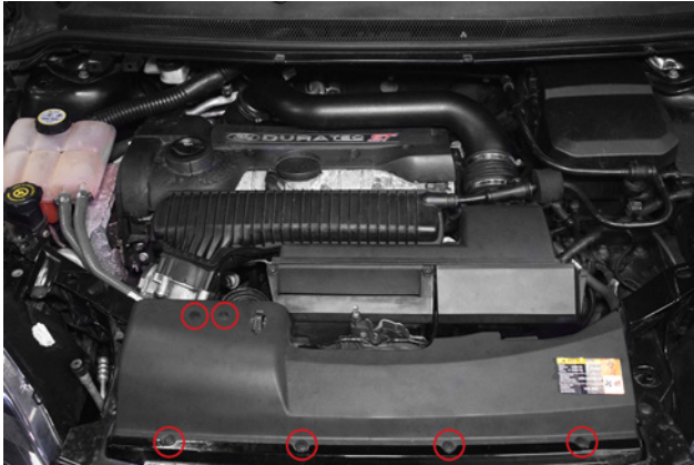
1. Remove 6x Philips trim screws on slam panel cover.
