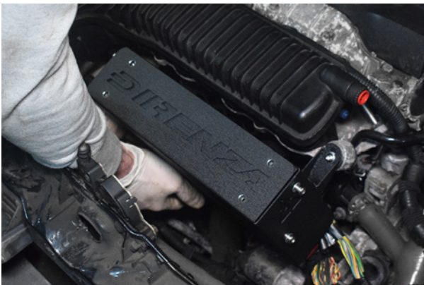
27. Slide the ECU cover into position.
