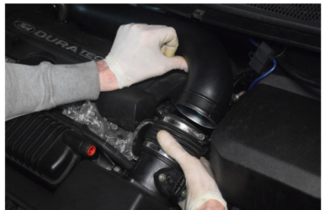
12. Remove connector pipe.
