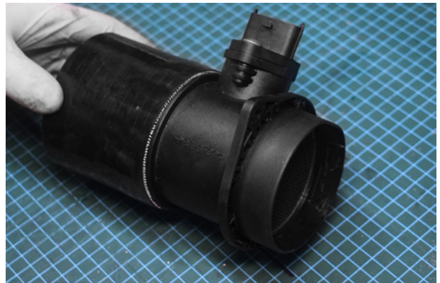
34. Install straight silicone onto the MAF. This can be done off the car.
