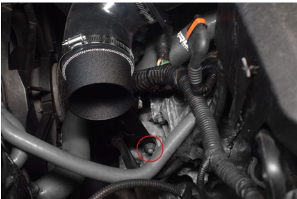
39. You can now fully tighten the lower bracket.
