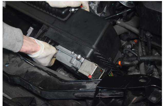
16. Our car has the security cage around the ECU.
