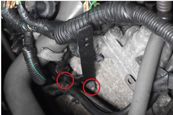
33. Step 32 Continued: Re-attach wiring fitting.
