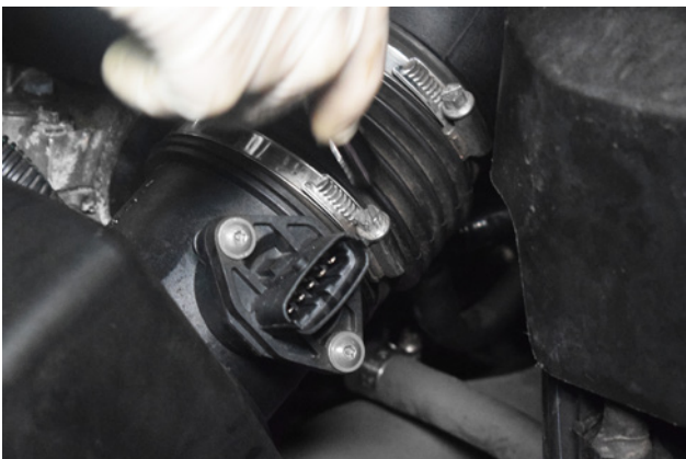
11. Remove two jubilee clips connecting Crossover pipe to MAF.
