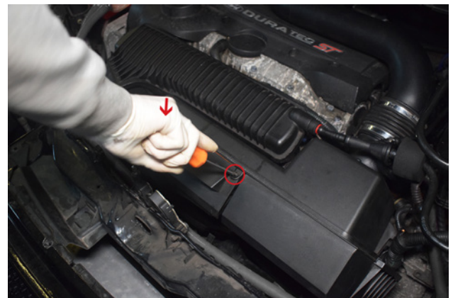
4. Remove 2x screws on Airbox.
