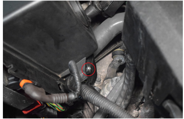
14. Remove T20 connecting wiring loom to air box.
