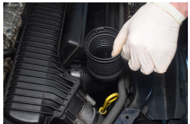
6. Remove air feed pipe.
