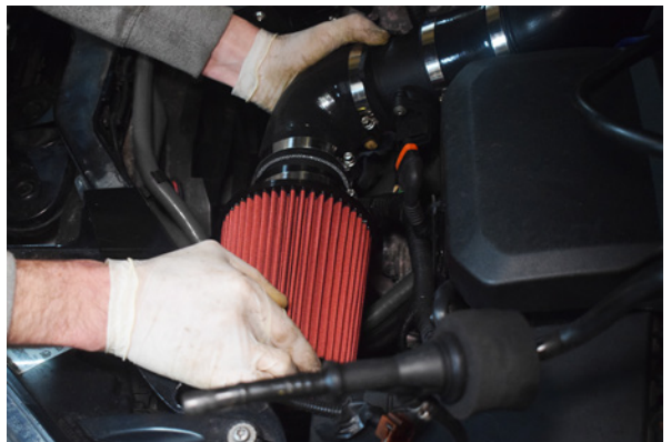
43. Slide Air Filter onto the end of the 90 degree silicone.
