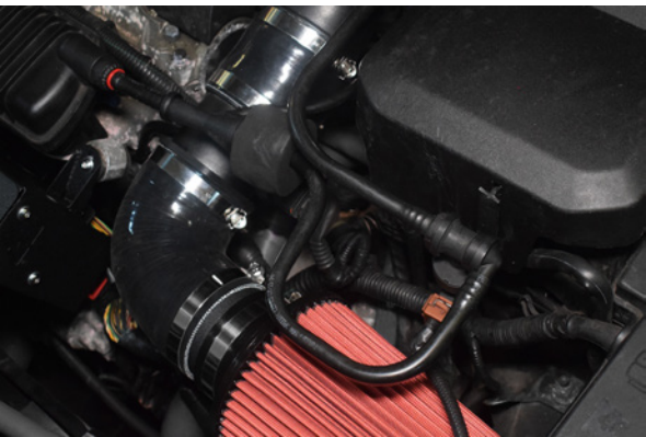
45. Re- Attach vacuum pipe and plug.
