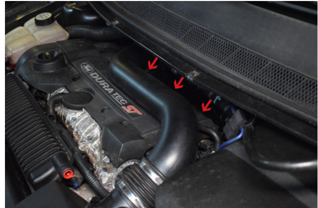
10. Loosen 3x 10mm bolts on cross over pipe to allow some move movement.
