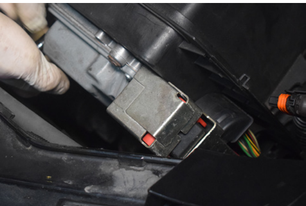
15. Depending on your model year, the ECU may have a security cage.
