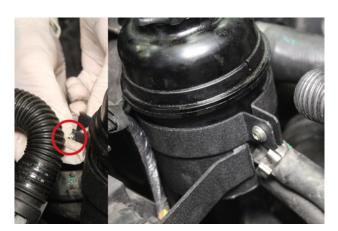
22. Place the power steering reservoir into the new bracket and tighten the clamp using the supplied allen bolt.
