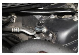
35. Use the second nut from the original AC bracket to secure and fit the new AC pipe and Direnza clamp.
