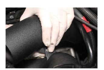
27. Secure the two hard pipes together using the supplied allen bolt.
