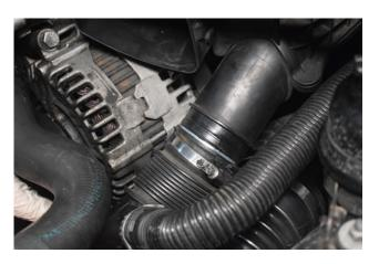
8. Undo the 6mm jubilee clip on the front induction feed and pull away.
