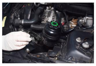
12. Take the reservoir out of the holder and remove the holder from the vehicle.
