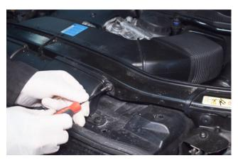
2. Remove 2x T20 securing the OEM air scoop.
