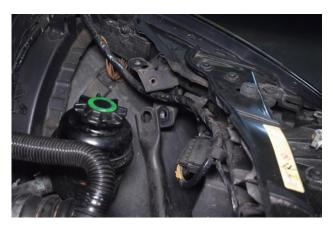
20. Remove the chassis brace.
