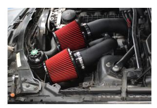
34. Fit the second filter to the front hard pipe and secure using the supplied jubilee clip.
