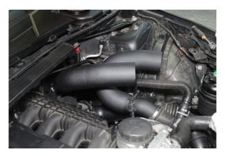
29. Secure the front hard pipe to the passenger side strut tower stud using the nut you removed earlier from the AC bracket.
