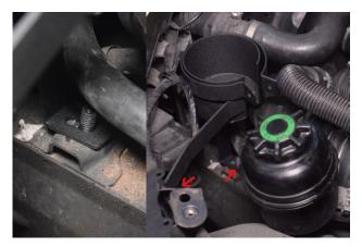
21. Place the new Direnza power steering reservoir bracket into position on the same studs the chassis brace uses.
