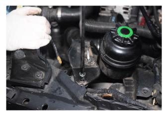
13. Undo 2x 10mm nuts on the second bracket..
