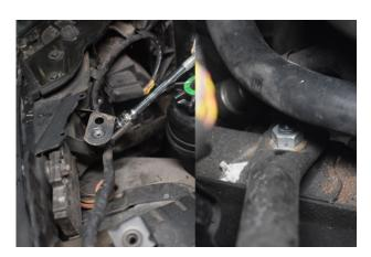
19. Remove the 2x 16mm nuts securing the chassis brace.
