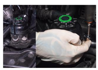
11. Remove the 2x 10mm nuts on the power steering reservoir and the 10mm bolt on the clamp.
