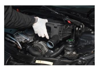
10. Lift up and remove the air box.
