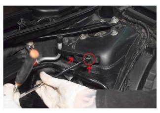
17. Remove the 2x 10mm nuts on the plastic bracket securing the AC pipe.
