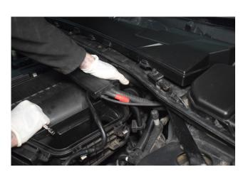
9. Undo the 6mm jubilee on the rear induction feed and remove.
