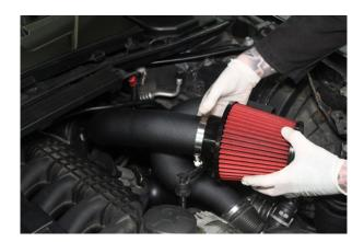
31. Place the first filter over the rear hard pipe.
