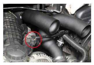
30. Push vacuum pipe back into position ensuring the pipe goes underneath the two hard pipes.
