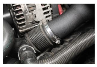
28. Tighten 2x jubilee clips connecting the two hard pipes to the OEM induction pipes.
