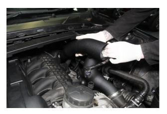
26. Install the rear induction hard pipe.
