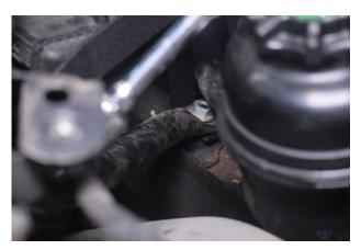
23. Re-install the chassis brace and tighten 2x 16mm nuts.
