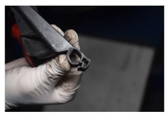
18. Un-clip the bracket from the AC pipe.
