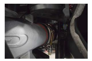
34. Place all necessary clamps in position before installing hot side boost pipe.
