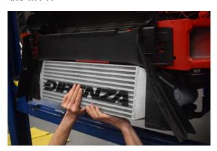
30. Lift MVT intercooler into position, ensuring it is sitting securely on all mounting and guide points.
