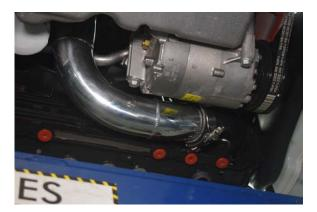
43. Install cold side boost pipe into the silicone joiner you have placed onto the throttle body and 90 degree silicone.
