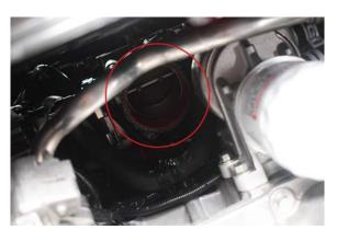
41. Place largest silicone joiner onto the throttle body.
