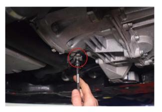
18. Remove 2x 10mm nuts on hot side boost pipe support brackets. We have circled one, follow the pipe to locate the second.
