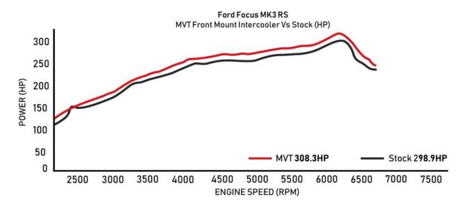
Without any engine remapping, the Focus RS fitted with Direnza's MVT intercooler makes 308.3bhp, thats 9.4 more than standard. With a torque reading of 338.4FtLb thats 6.3 FtLbs gained. A fantastic upgrade for a bolt on part which offers even more potential gains if combined with a remap.
