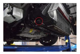
25. Use 8mm socket to remove 2x bolts on lower intercooler brackets. (One each side of the OEM intercooler).
