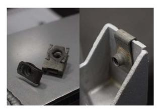
27. Take metal clips from the OEM intercooler and place them onto the equivalent position on the MVT.
