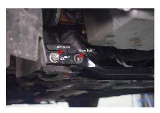
17. From underneath the car, remove 2x 15mm bolt and 2x 18mm nuts on the chassis brace and remove.
