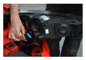
4. Disconnect plug on the back of both headlights and remove the lights.
