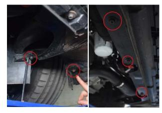
11. Remove 7x screws on front edge of bumper holding on the bumper undertray.
