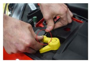
52. Ensure the bonnet safety catch is connected before closing the bonnet!
