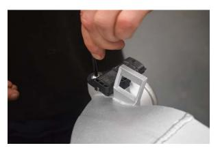
28. Remove OEM MAP sensor from the stnadrd intercooler and place into the MVT intercooler. Use supplied hardware to secure it.
