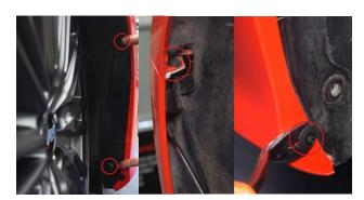
7. Under wheel arch, remove 2x T30 Torx and 2x trim clips. Repeat this on both sides.
