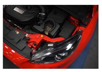
2. Remove the 2x T30 on each headlight unit.
