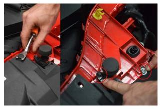
6. Remove 5x screws across top panel & 2x push clips.
