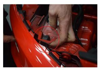
15. Lift clip and push down and rubber stop on the top of bumper, located on the drivers side.
