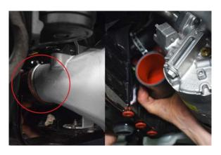
42. Put 90 degree silicone joiner onto the cold side End tank.
