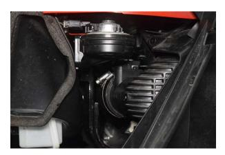
21. Move onto the cold side boost pipe and loosen 2x 7mm jubille clips.
