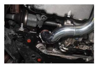
36. Lift boost pipe into position, Secure this pipe to the turbo using supplied clamps.
