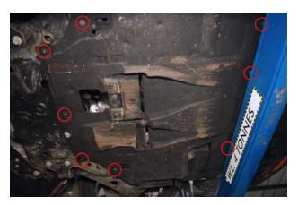
9. Remove 8x Torx on the engine undertray. There are also 2x clips to remove.
