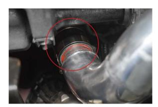
35. Place the smallest silicone joiner onto the hotside boost pipe, to be connected to the turbo.
