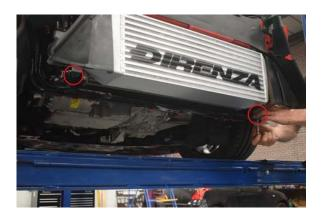
31. Secure the MVT in original position using 2x 8mm bolts.
