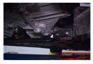
45. Re-install chassis brace by reversing step 17.
