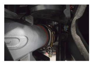
33. Install silicone joiner on the hot side end tank (1 of 3 joiners the same size).
