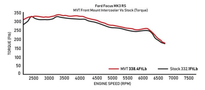
Track tests on the intercooler showed temperatures to be upto 8.4 degrees lower than standard. The lower outlet tempratures provide better performance whilst also protecting the engine. The pressure drop across the intercooler was also 0.62psi lower than standard. This means the Turbo doesn't need to work as hard to produce the same amount of boost.
