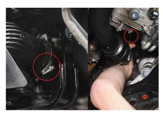
19. Loosen 2x 7mm jubilee clips on hot side boost pipe. One is located near the end tank and one near the turbo.
