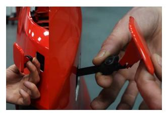
5. Use pick to remove washer jet. Lift and roll upwards to release. Do this on both sides.
