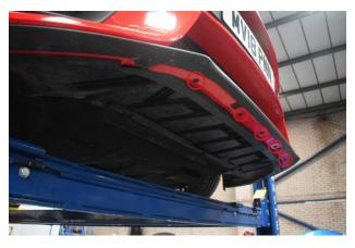
8. Remove 7x plastic screws from the underside of the bumper. You can use the trim tool to help pull these out.
