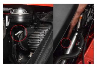
22. The jubilee clips are located near the outlet on the end tank and on the throttle body.
