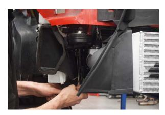
29. You can loosen radiator support brackets (2x 10mm per side) to help fit the MVT.
