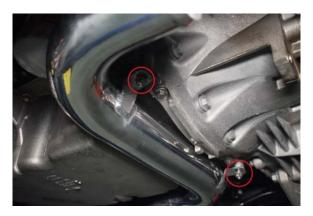
37. Re-install nuts on the hot side boost pipes support brackets.
