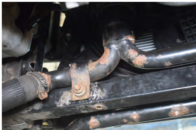
10. Undo 5x 10mm bolts from both the front and rear Y pipes and clamps from both hot side and cold side of intercooler hoses.
