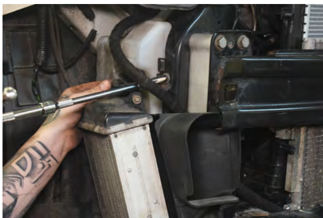
7. Undo 10mm bolt to remove intercooler bracket. (Drivers side RHD)
