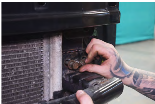
15. Remove the lower crash bar.
