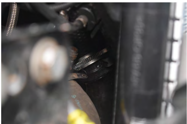
12. Loosen 7mm jubilee clip on top boost hose and remove from turbo. There is a handy gap underneath the headlight for access.
