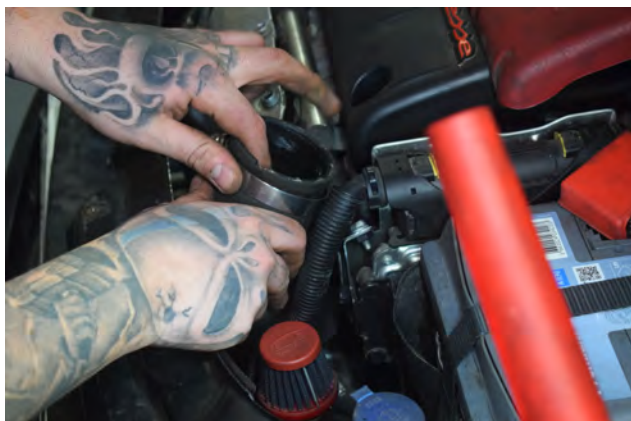
13. Also loosen 7mm jubilee clip on throttle body inlet hose and remove.
