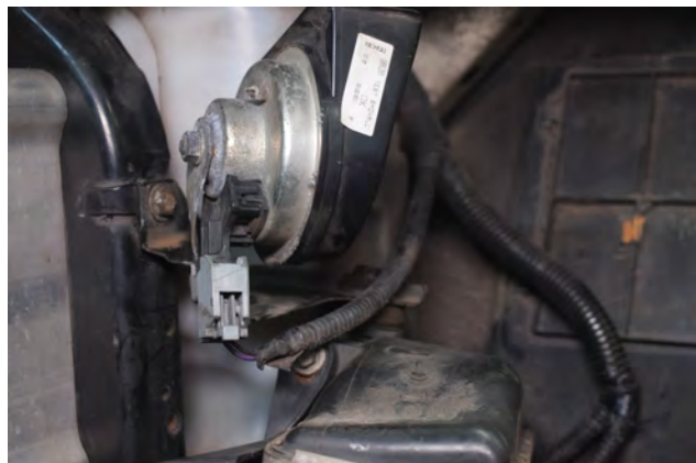
9. Intercooler bracket on the passenger is also used for the horn, place the horn in a safe place until later.
