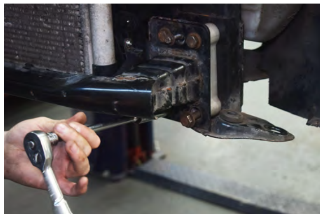
14. Remove 4x 17mm bolts and 1x 10mm bolt holding on lower crash bar. Repeat this on both sides.
