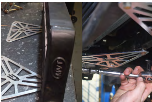
16. Place intercooler support brackets onto the MVT Intercooler and use the supplied 2x 13mm bolts to secure into place. Use 4x10mm bolt (from underside of bumper) to mock up the intercooler in the correct position.
