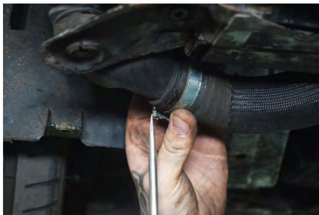
8. Remove 2x hose clamps from the OEM intercooler hoses. The intercooler can then be removed from the Y pipe. (Repeat steps 7 & 8 on both sides).
