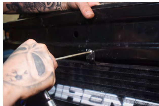
18. Once drilled, secure the MVT to the upper crash bar using the 4mm allen bolt, nut and washer.
