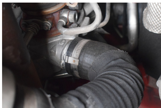
41 Undo jubilee clip securing pipework to the turbo.
