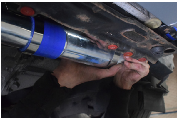
67. Insert the last piece of hard pipe between the two silicone joiners and secure all jubilee clips.
