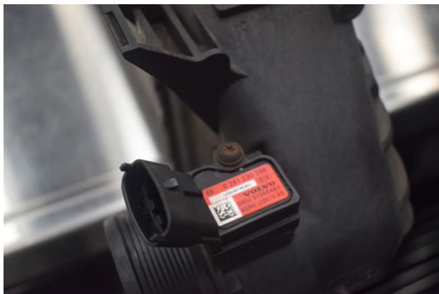
49. Remove the sensor from the OEM intercooler by undoing T20 screw.
