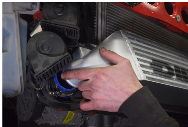
52. The MVT intercooler can now be lifted into position.
