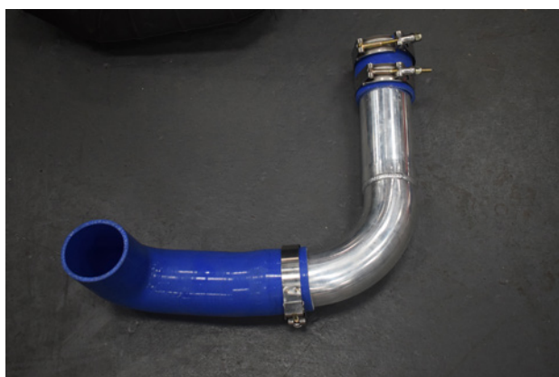
47. The new cold side pipework should look like this.
