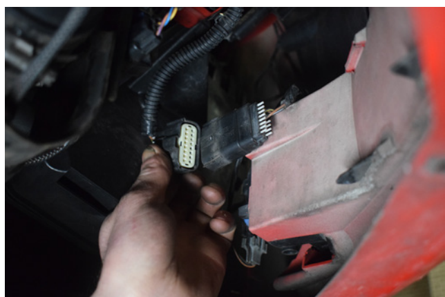
21. Unplug front bumper wiring loom located on the passenger side of the car.
