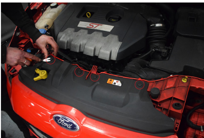
8. Remove the 4x plastic trim clips on the plastic slam panel cover.
