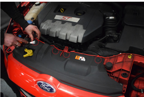
81. Install 4x plastic trim pieces on the slam panel and 2x T30 screws at each end.
