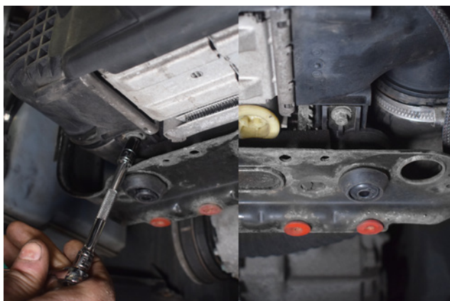
31. Undo 2x 8mm bolts securing the intercooler to the rad pack.
