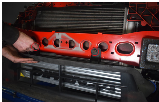
71. Install lower duct using original hardware.
