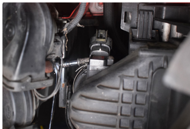
28. Undo jubilee clips connecting the intercooler to the cold side pipework.
