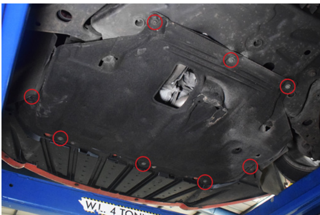
12. Undo 8x screws on the fabric engine undertray and remove from the car.
