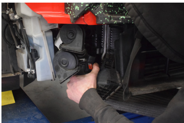
32. Lift and title the intercooler to remove from locating tabs and release from intercooler pipework.
