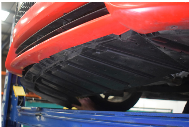
19. The bumper under tray can now be removed.
