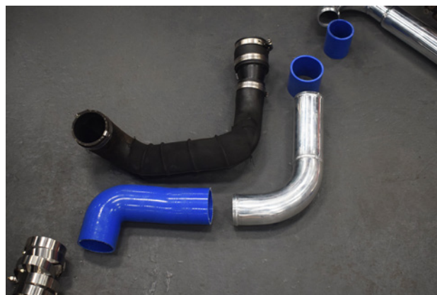
46. It is always a good idea to compare the original pipework with the MVT kit for reference.
