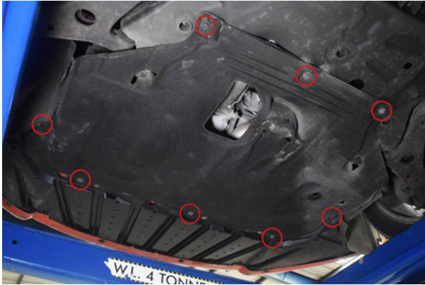
79. Fit engine undertray and secure using 8x screws.
