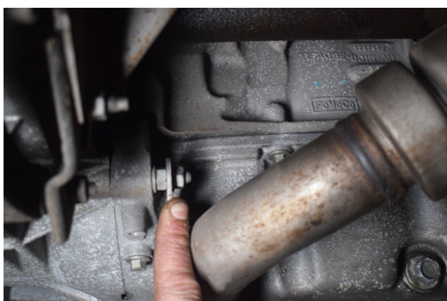
39. Remove 13mm nut on intercooler pipework bracket.
