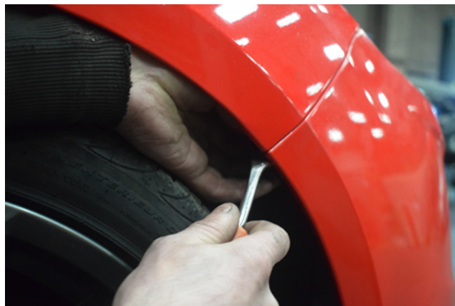
23. There is also 1 trim clip per side that needs to be removed from the inner wheel arch. (Pictured at step 24).
