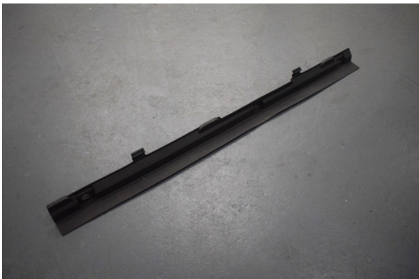
80. Fit plastic diffuser lip using 3x Torx.
