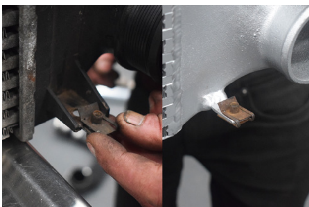
51. Remove 2x spire clips from the original intercooler and install on to the MVT.
