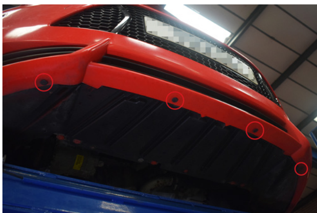
13. Remove 6x plastic trim clips from underneath the front bumper.
