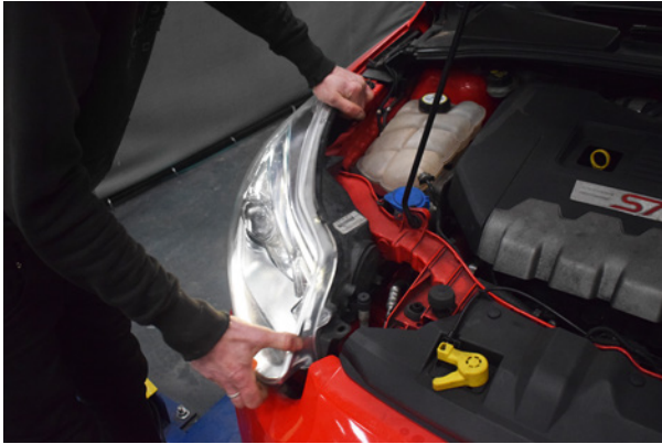
85. Install the headlights, once seated in the correct position.
