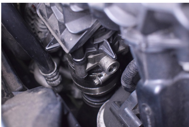
44 Undo jubilee clip securing the cold side pipework to the throttle body.
