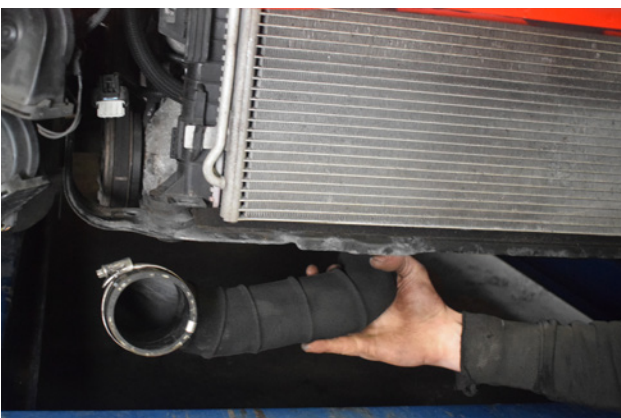
45. The cold side pipework can now be removed from the car.
