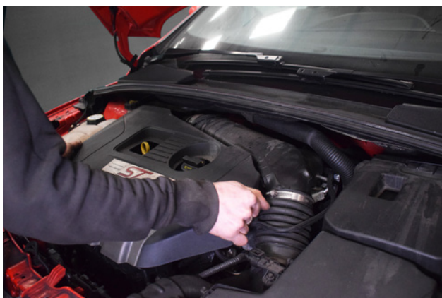
43. Lift and pull engine cover to remove. This allows slightly better access to the the throttle body.
