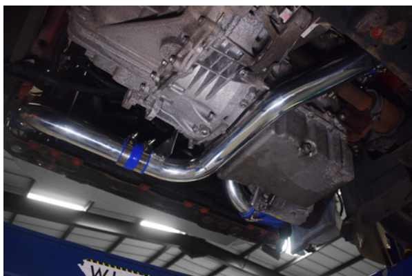
68. Your intercooler and pipework has now been installed.
