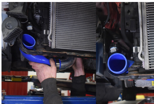
48. Lift the new cold side pipework into position on the car. At this point you can nip up the throttle body connection to avoid the pipework falling out of position.
