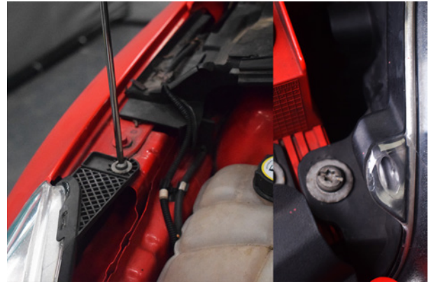
86. Secure the headlights using 2x T30 screws. Do this for both sides.
