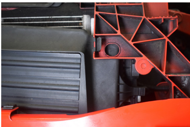
37. Remove the flap control panel by sliding and lifting out of position.
